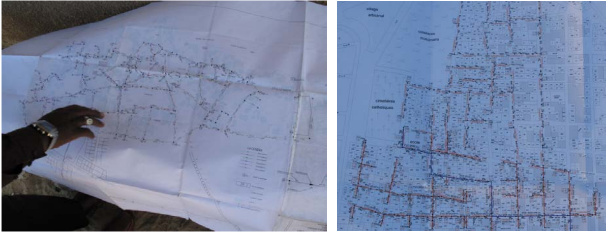
Left: Section of the (very winding) layout of the Ngor sewer route, Dakar. Right: Section of the (more regular) layout of
