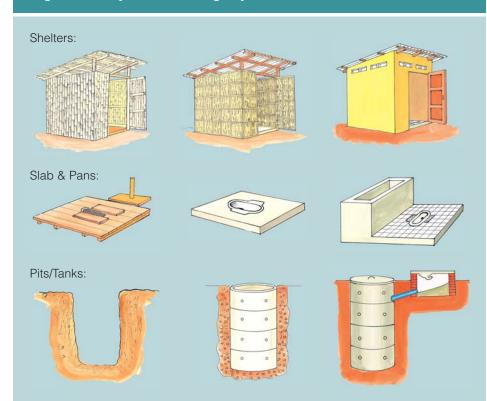
Latrines have essentially three components and can be constructed with any combination of the options for: (1) an above-the-ground shelter mainly for privacy, (2) a latrine slab which incorporates the latrine pan or hole, and (3) the below-the-ground structure into which the waste is passed.
