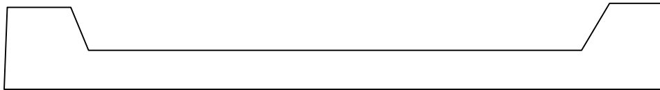
Figure 1: Concrete mixing pad (made from concrete)
