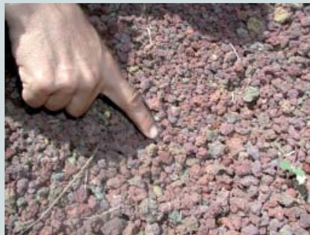
The volcanic filter material ( hormigón rojo ) used for constructed wetlands in Central America. Source: Martin Gauss, 2006.
