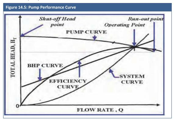
The performance curves reflect standard testing. Pump manufacturers typically calculate performance curves using a pressure gauge and a flow meter connected to the discharge port. For any anticipated total head, the discharge capacity can be determined. Pump performance curves are available for each pump model.
