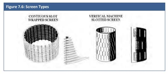
While a screen is the more expensive alternative, it is necessary if the aquifer is composed of loose material such as fine sand, gravel or soft sandstone. A slotted or perforated casing can be used when the aquifer formation is more consolidated, such as hard sandstone or fractured shale.
