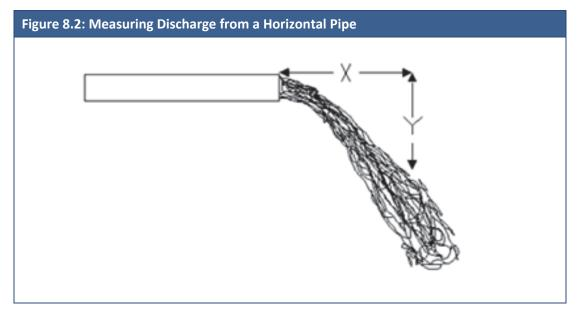
The following describes the procedure for measuring flow from a horizontal pipe as shown in Figure 8.2. Two conditions must be met for this procedure to work:
