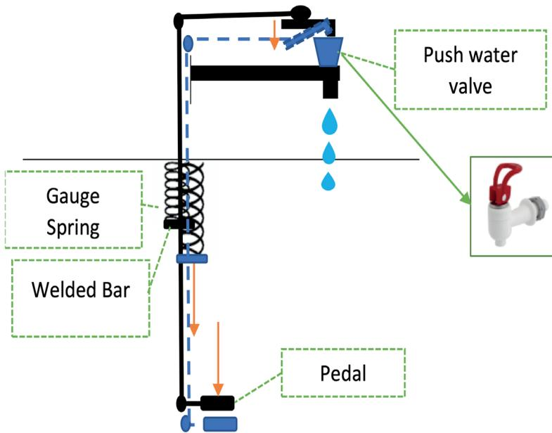
▲ Direct action arrangement schematic diagram.
