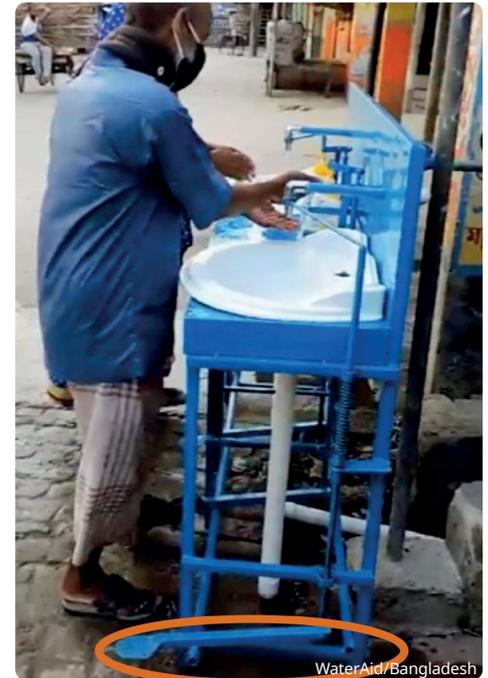
▲ A pedal arrangement working in an upward direction. Note the lift cock is getting direct upward push for water distancing.
