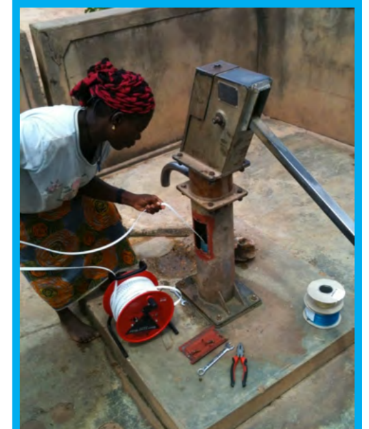
A community woman using a level logger to assess the water level of a borehole
