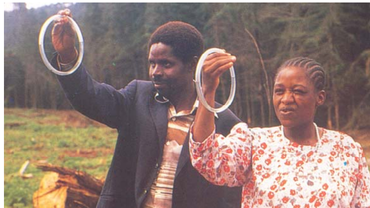
Two farmers are using circular transparent hosepipes filled halfway with water to sight horizontal lines.
