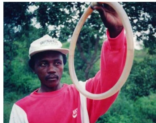
Sighting along the two water levels in a circular transparent hosepipe filled halfway with water, gives an exact horizontal line.
