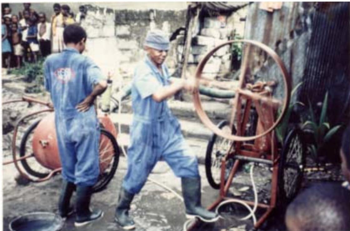
Picture 3 Compared to traditional emptying MAPET has improved the hygiene on the compound and the working conditions for the emptiers.
