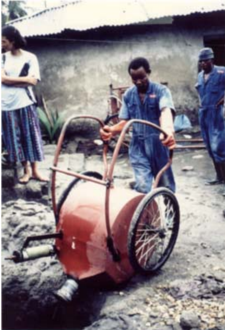
Picture 4 On-site disposal in a dug hole on the customers' compound, by tipping the 'Kibuyu'
