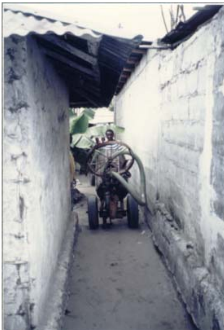
Picture 2 The equipment is small scale, a requirement for access to full pits in unplanned areas.
