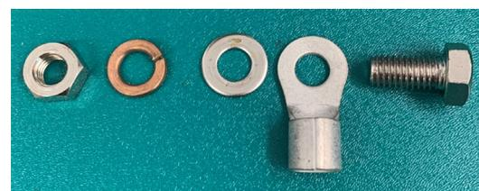
Use insulated tools when tightening the nut. An accidental battery short circuit can be very dangerous, and the currents can melt your uninsulated spanner, or the spark can cause a battery explosion.
