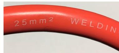
Be aware that some cables can have very thick insulation and they may appear thicker than they are. Find out the actual core diameter by looking at the cable marking or at its specifications, or alternatively do a physical check. Strip a bit of cable insulation away and look at the copper core of the cable and estimate the core diameter.
