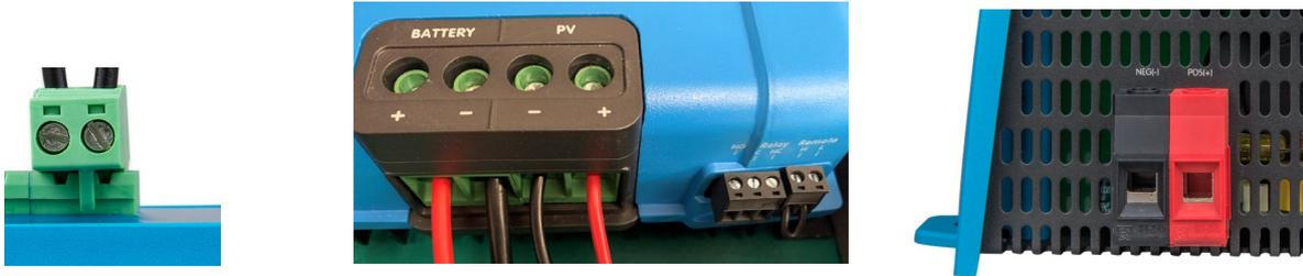
Strip a sufficient length of cable insulation before inserting the bare end into the connector cavity. Avoid cable insulation entering the connector. This can lead to too much resistance and the connector will heat up and potentially melt. Avoid uninsulated cable (bare cable) to be visible outside the connector. This is dangerous it can cause electrocution or a short circuit.
