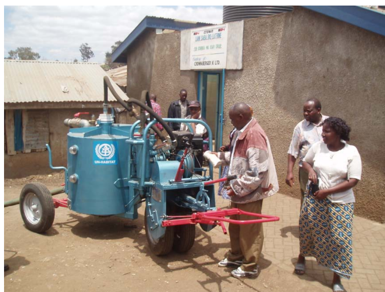
Figure 3.9: The 'vacutug' developed by UN-Habitat.
