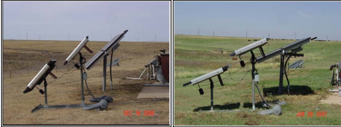
Figure 6 – Solar panel tilt angles: winter tilt with more angle from horizontal [left] and summer tilt with less angle from horizontal [right]. (Source: “Renewable Energy Primer-Solar.”)
