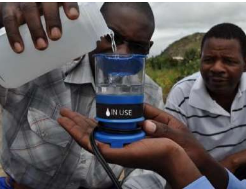
Figure 9. MSR SE200 community chlorine maker (Source: PATH)
