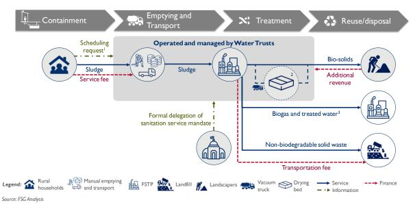
Notes: 1. Households can contact either LWSC or the Water Trusts; 2. The drying beds were located at a different location in Kanyama due to land availability issues; 3. Biogas and treated water are consumed on-site; Sources: ISF-UTS and SNV. 2021. Anaerobic Respiration for Faecal Sludge Treatment and Reuse; FSG interviews.
