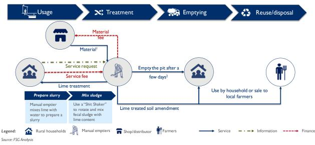
Notes: I. Material includes screw auger, PPE kit, and emptying tools; 2. The time after which the pit is safe for emptying is inconclusive as per existing research; Source: Conceptualized based on <u>iDE Cambodia Alternating Dual Pit upgrade model</u>.
