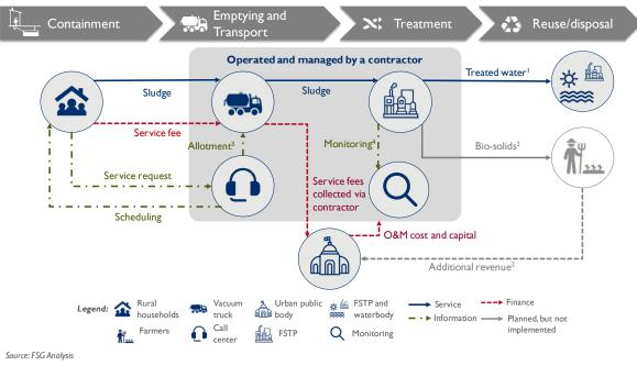
Notes: 1. Treated water used to irrigate land at the FSTP facility and recharge a nearby water body; 2. Sale of bio-solids was planned but not implemented; 3. Emptying jobs are allotted to either one of the two trucks; 5. CDD Society, a technical partner, monitors the FSTP for compliance with national effluent standards. Sources: Centre for Policy Research. 2020. Operation and Maintenance (O&M) Aspects of Faecal Sludge Management in Small Towns; FSG interviews.
