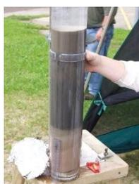
Fig. 1 Sediment core Sampler
