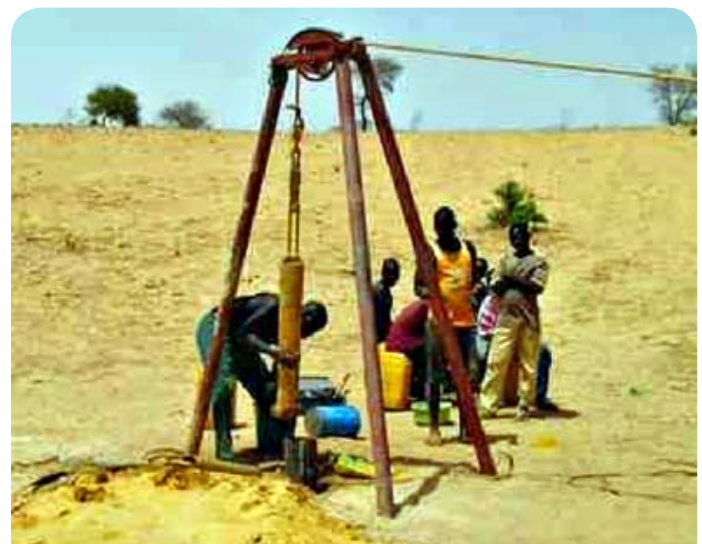
Fig. 2.16 Hand percussion rig in action
