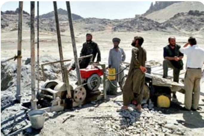
Fig. 2.7 Cable tool drilling, Pakistan
