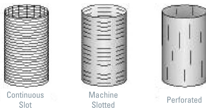
Fig. 2.42 Slotted screens
