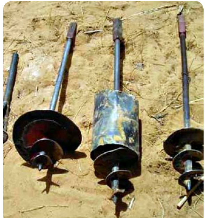
Fig. 2.15 Auger bits
