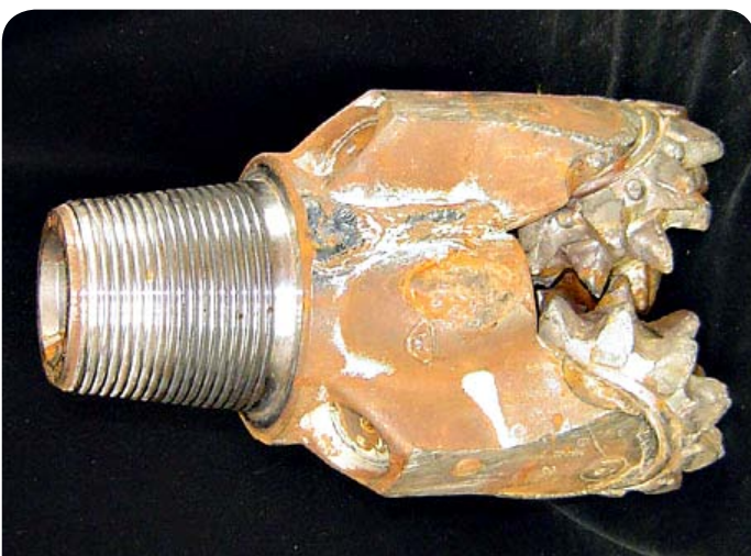
Fig. 2.67 Rock roller bit
