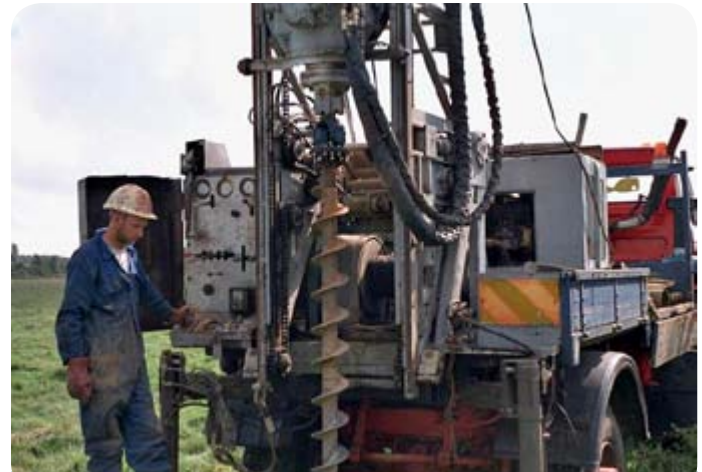
Fig. 2.6 Auger drilling
