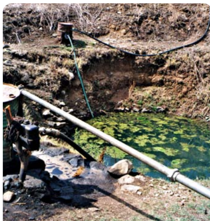
Fig. 3.16 Spillage from a diesel pump
