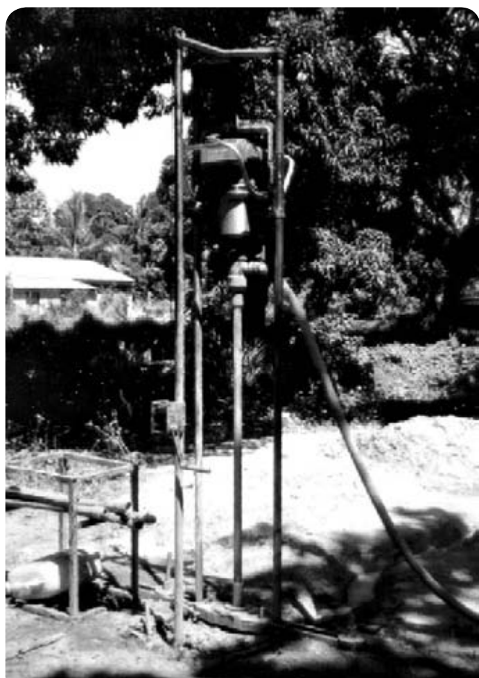
Fig. 2.61 Small rig with petrol engine drive, Tanzania
