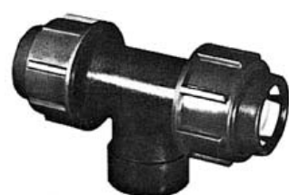
L) Tee 90° (2 x female compression fittings and 1 x threaded female socket for GI-pipes)
