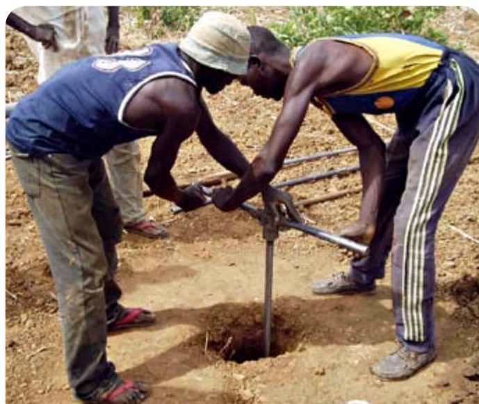
Fig. 2.14. Light hand auger equipment
