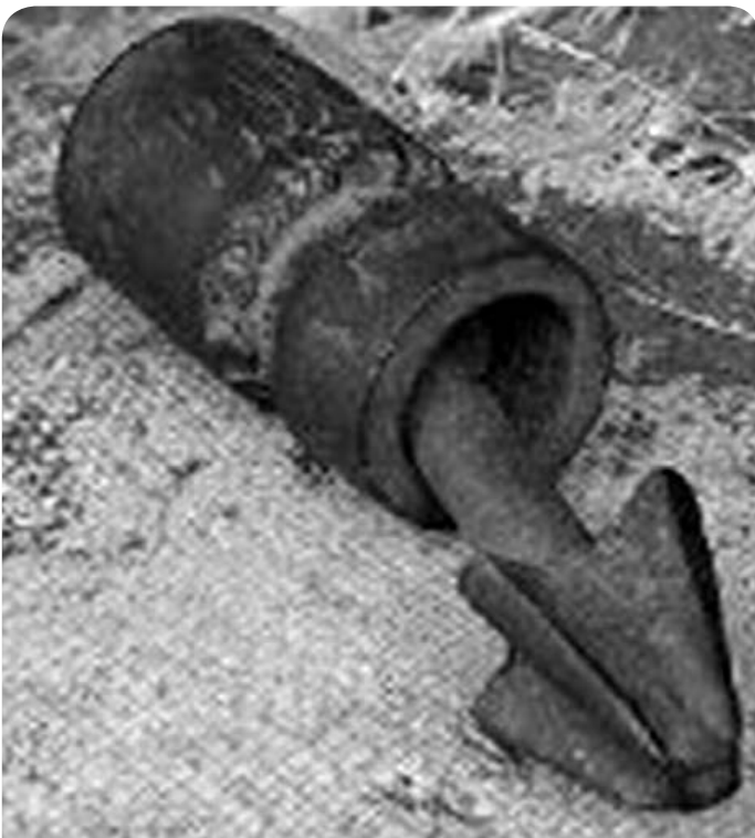
Fig. 2.25 Drill bit with footvalve above
