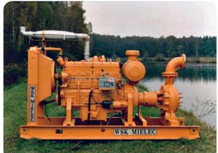
Fig. 4.18 Centrifugal pump, diesel driven © WSK
