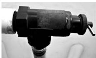
A) Pressure relieve valve, threaded male connection for GI or UPVC pipe
