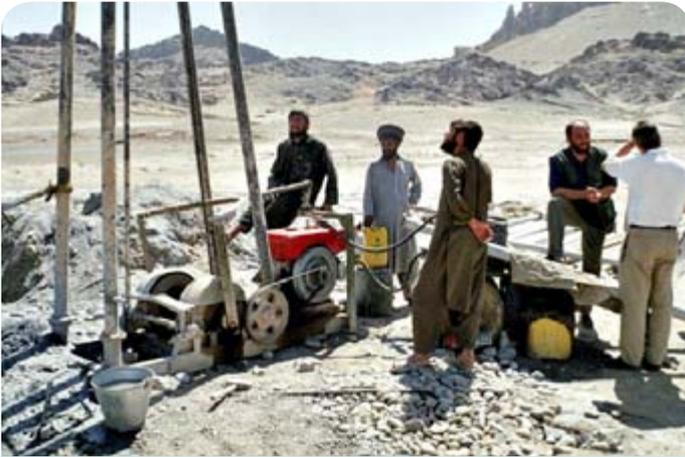
Fig. 2.7 Cable tool drilling, Pakistan
