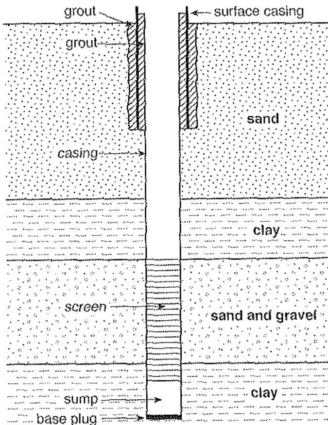
Fig. 2.36 Open borehole in unconsolidated formation © ITDG
