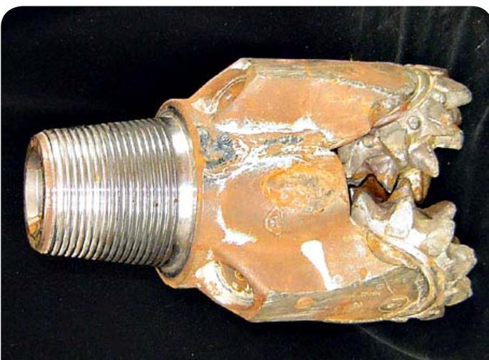
Fig. 2.67 Rock roller bit
