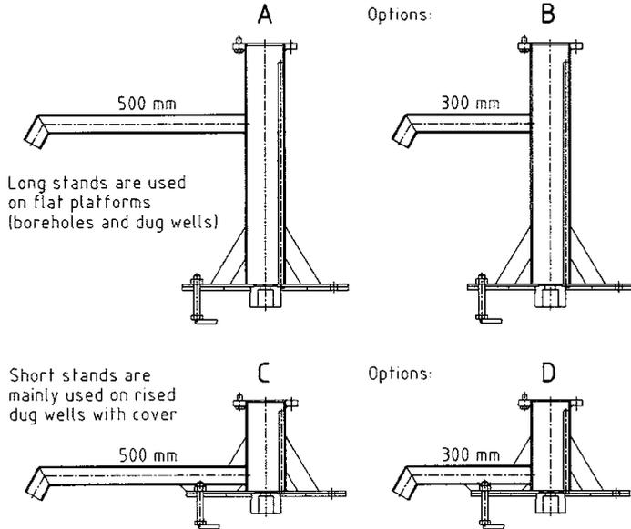
Long stands are used on flat platforms (boreholes and dug wells)
