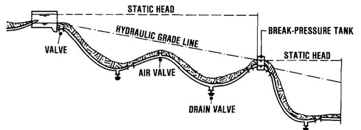
Fig. 4.23 Pressure pipeline © Skat
