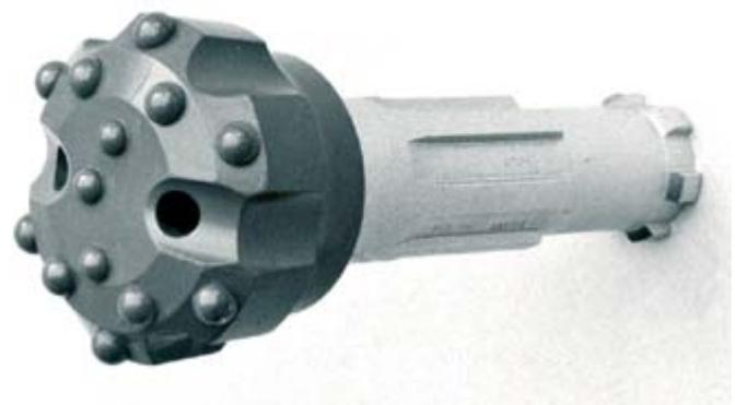
Fig. 2.68 Down-the-hole hammer
