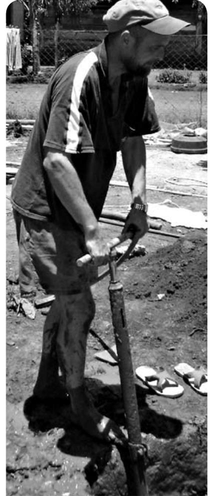
Fig. 2.33 Hand-operated mud pump
