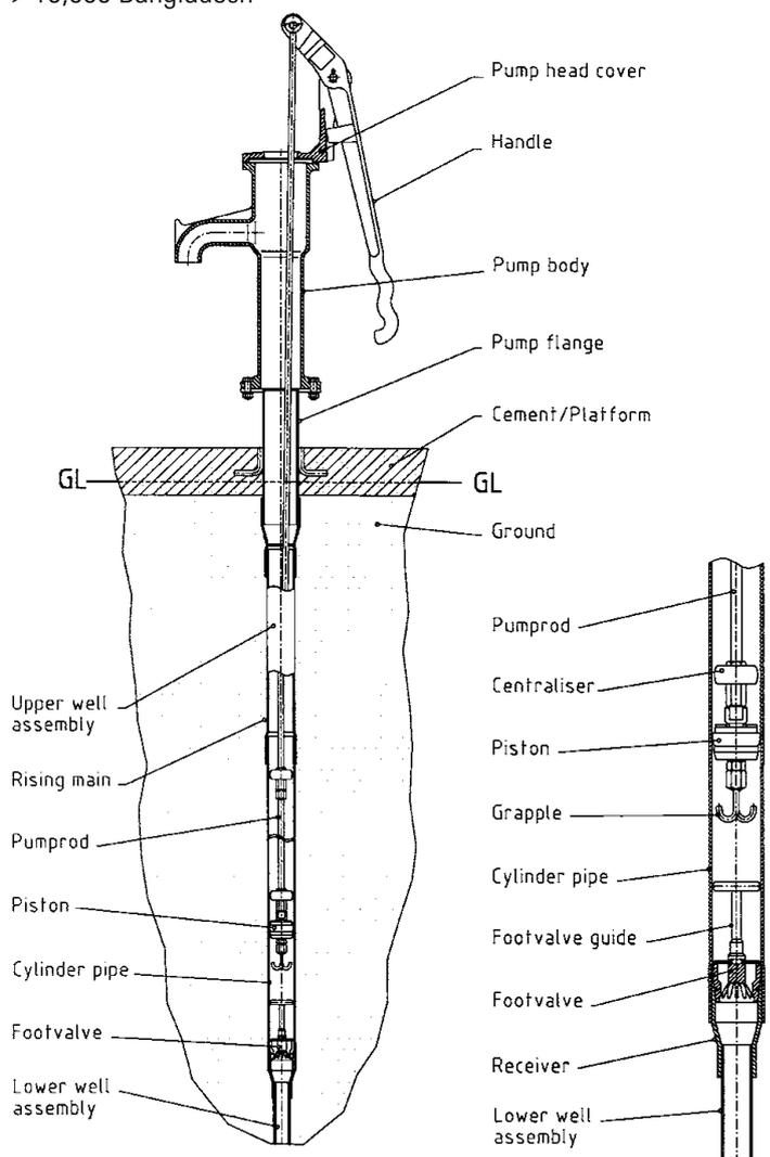
Fig. 1.26 Jibon pump assembly
