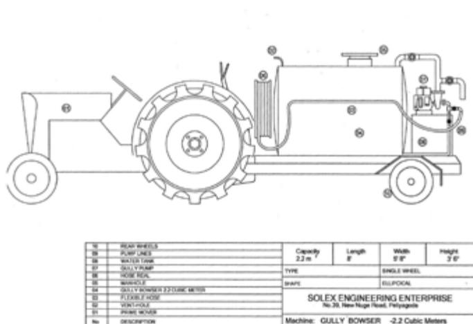
Fig. 5.8 Components of the Sri Lankan tractor-drawn trailer-mounted vacuum tanker © UNICEF Sri Lanka
