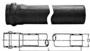
A) UPVC pipes with rubber ring joint
