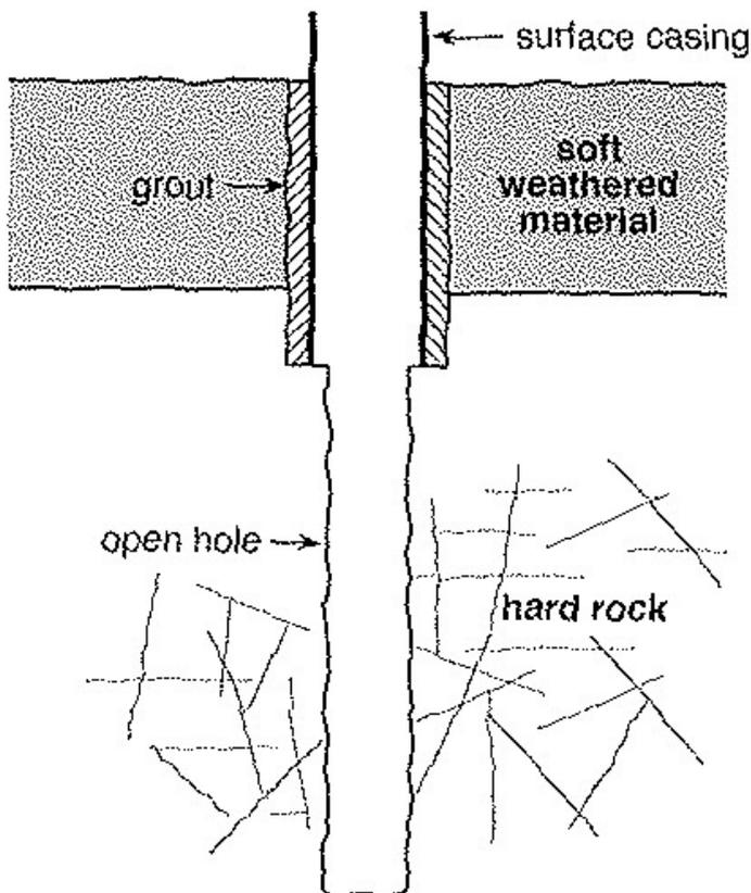
Fig. 2.38 Open hole in consolidated formation © ITDG
