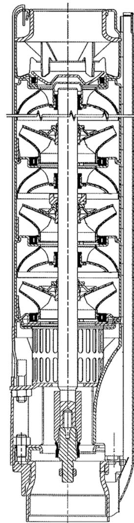
Fig. 3.13 Centrifugal pump
