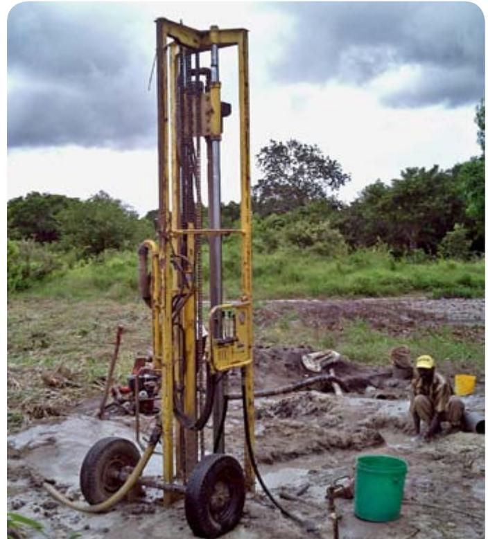
Fig. 2.9 Mud drilling, Tanzania
