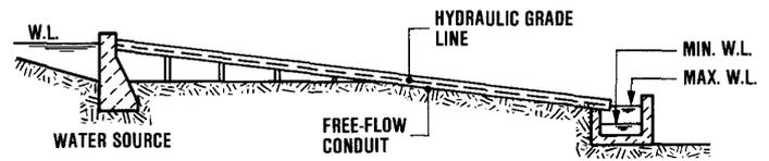
Fig. 4.22 Free flow pipeline © Skat
