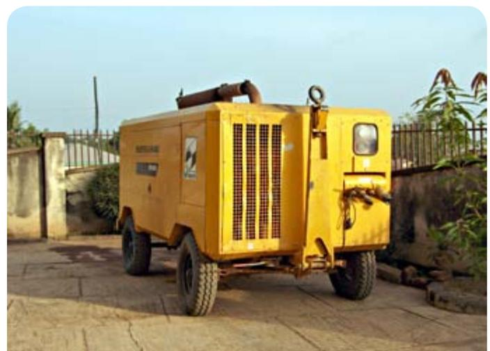
Fig. 2.63 Trailer mounted compressor, Nigeria
