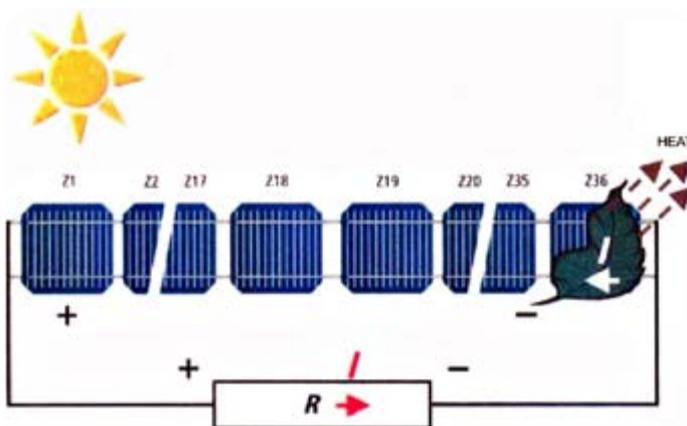
Fig. 3.8 Effects of shading © Skat
