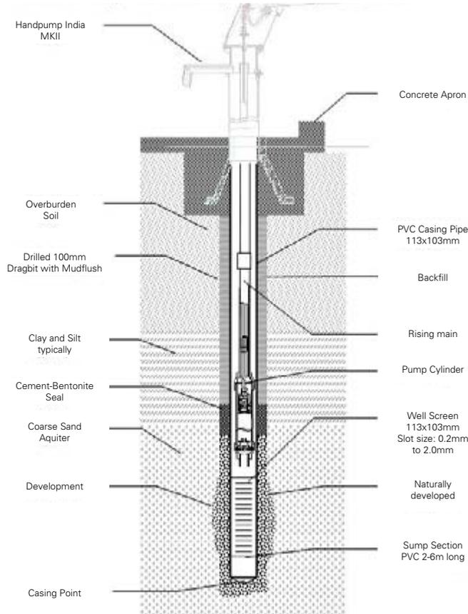
Fig. 2.57 Typical design drawing of borehole in unconsolidated formation with casing
