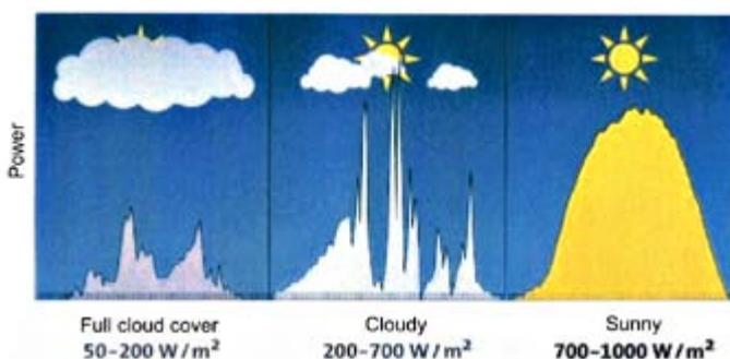
Fig. 3.5 Solar radiation
