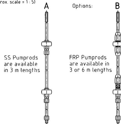
Fig. 1.44c Options for the U3M pump
