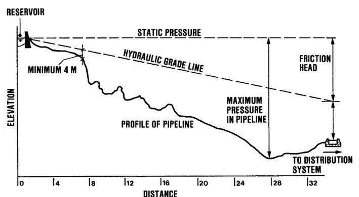
Fig. 4.24 Minimum pressure gradient © Skat
