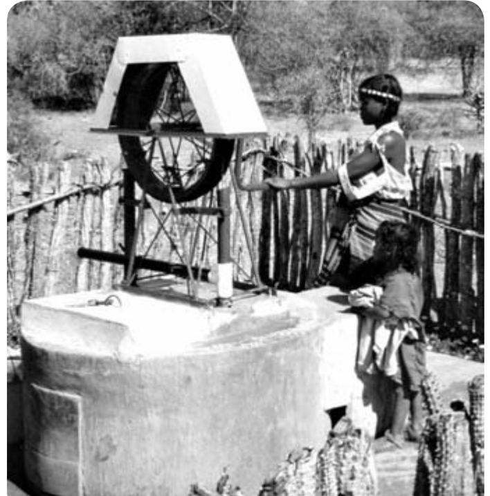
Fig. 1.14 Nicaragua rope pump
