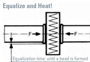
When jointing pipe ends together, a flat heating element is used instead of a bush and spigot. The force (F) required for pushing the pipe ends towards the heating element is approximately 0.01N/mm<sup>2</sup>.
