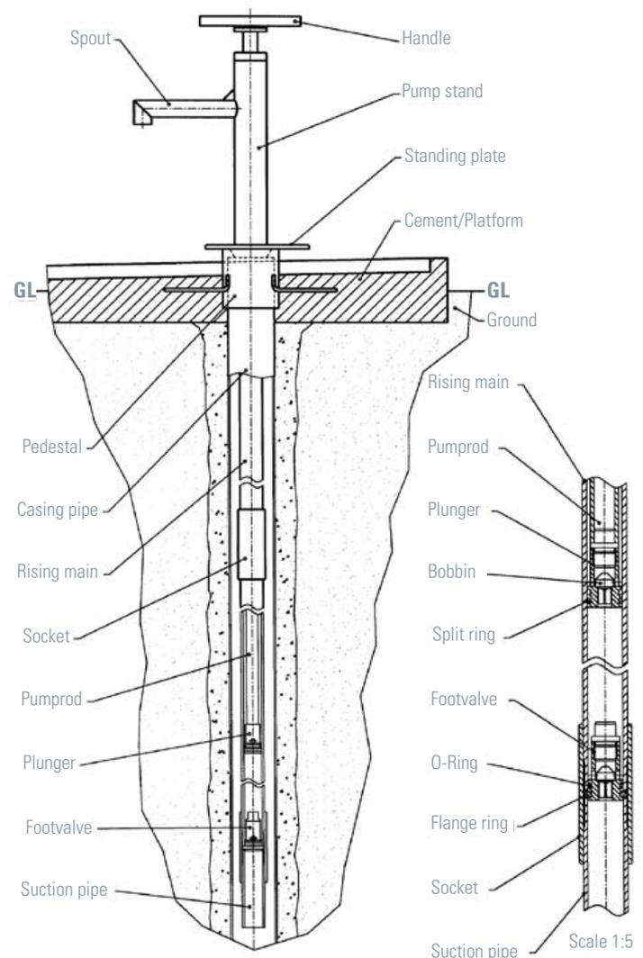
Fig. 1.21 Malda pump assembly
