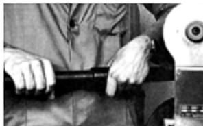
Note that only pipes and fittings up to a diameter of 65 mm (2 1/2") should be joined by hand. For larger sizes, special guiding equipment is required.
