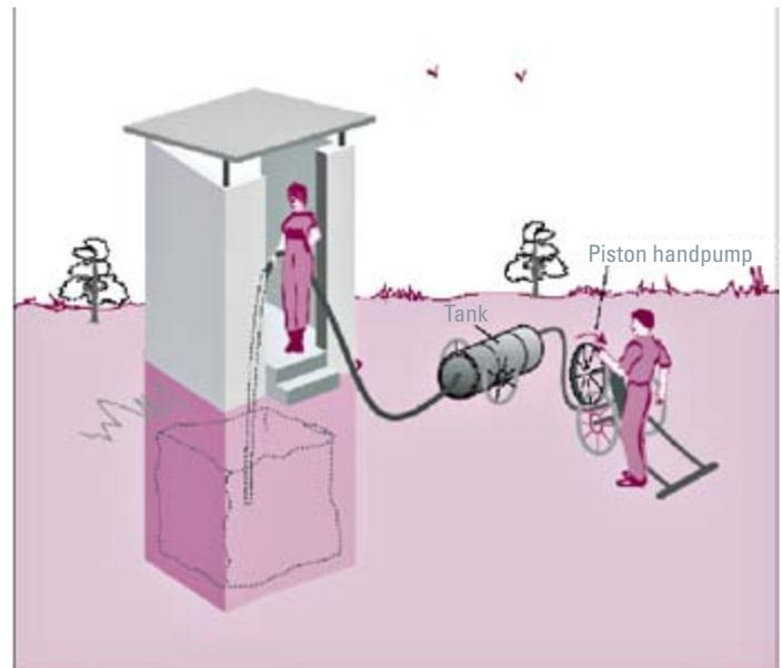
Fig. 5.3 The MAPET system
