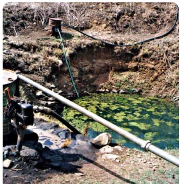
Fig. 3.16 Spillage from a diesel pump
