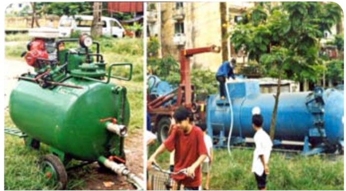
Fig. 5.6 Mini tug and storage tank, which can be hook-lifted and hauled away
