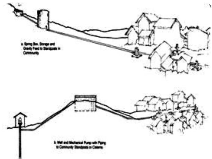
Fig. 4.19 Water transmission
