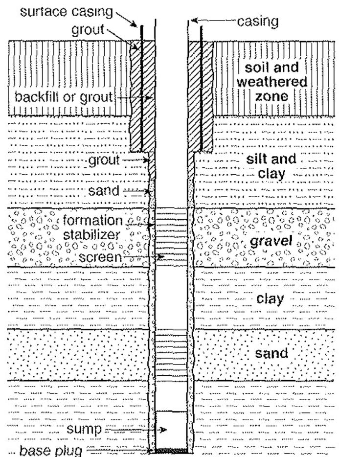
Fig. 2.35 Cased borehole in unconsolidated formation © ITDG
