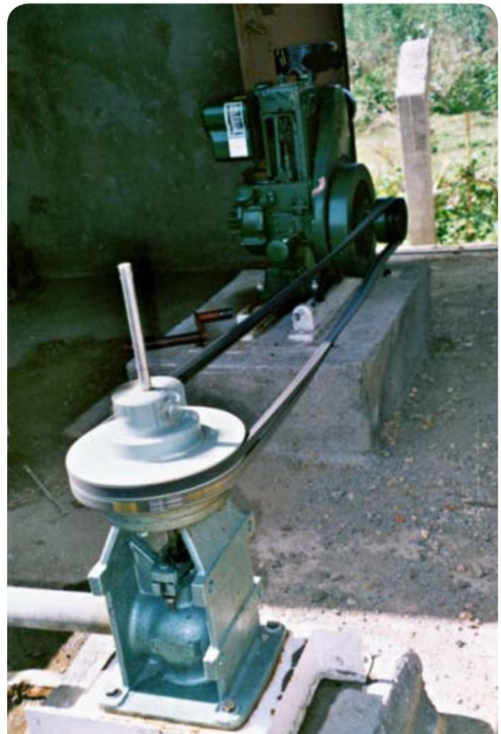
Fig. 4.16 Progressive cavity pump, Eritrea
