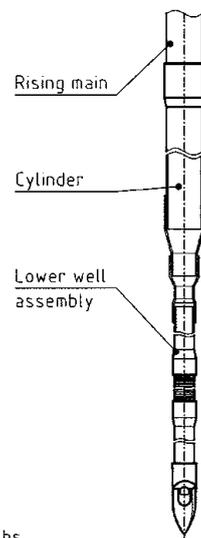
Fig. 1.26 Jibon pump assembly
