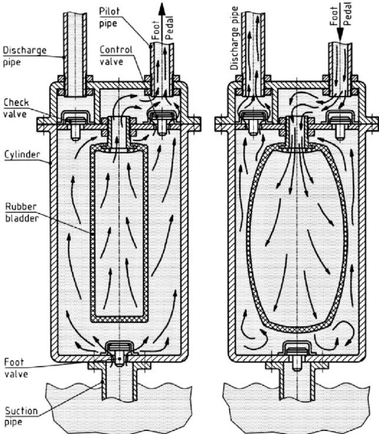
Fig. 1.8 Diaphragm pump
