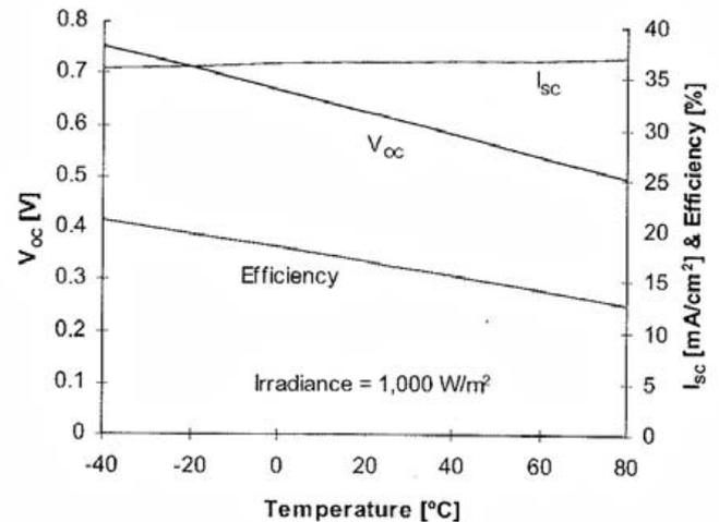
Fig. 3.6 Performance of mono-crystalline silicon cells © Skat
