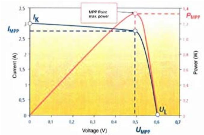
Fig. 3.7 Voltage-current characteristics of a solar cell © Skat
