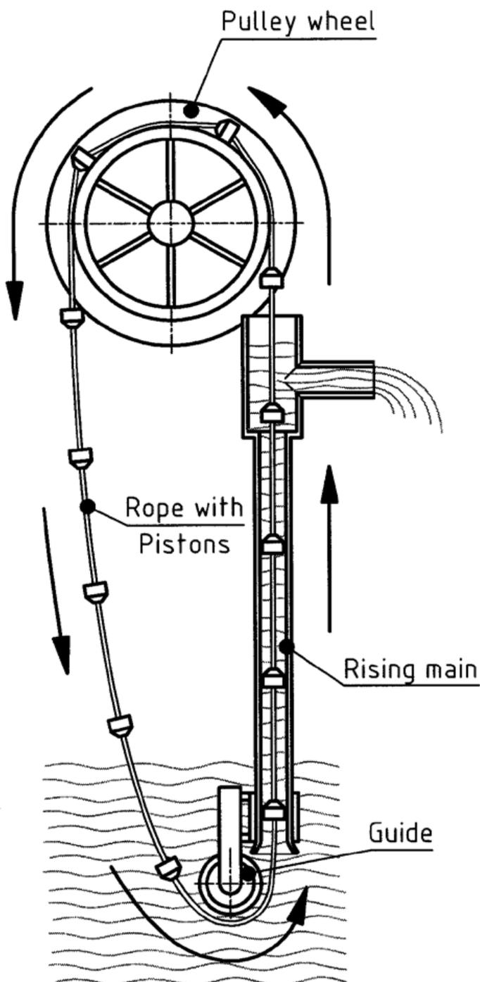
Fig. 1.5 Rope pump
