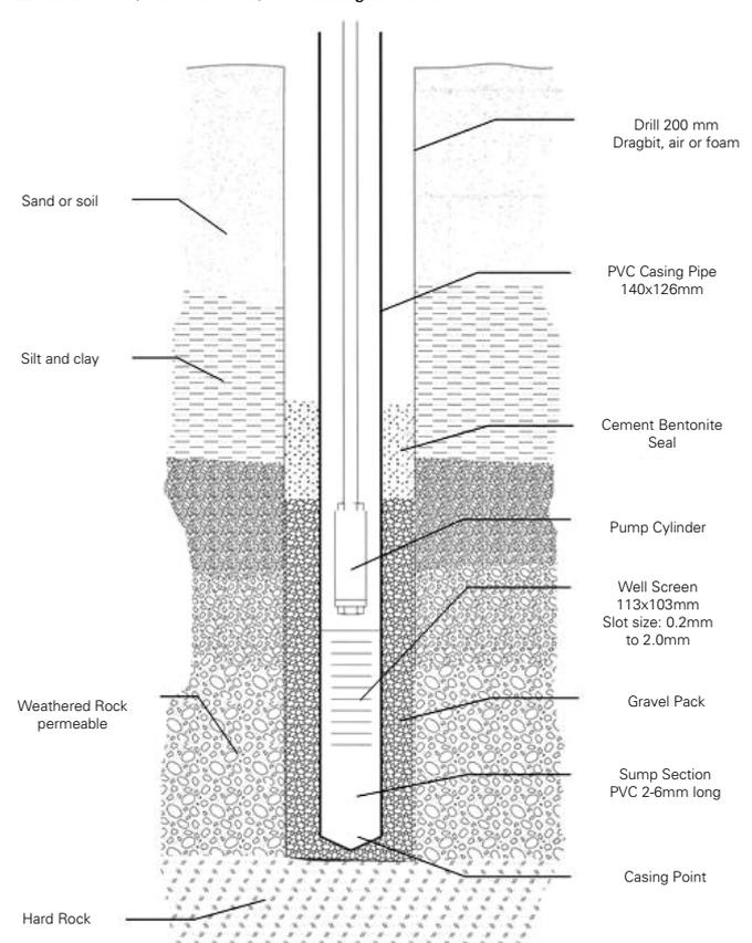
Fig. 2.60 Typical design drawing of regolith borehole
