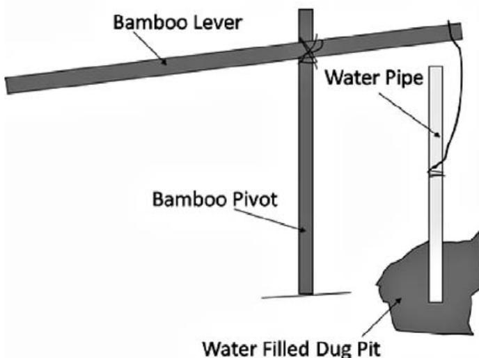
Fig. 2.22 Sludging equipment
