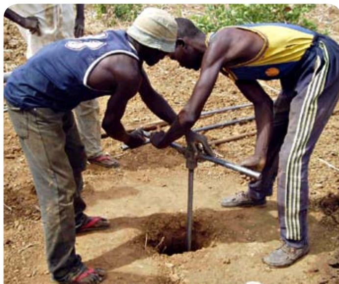
Fig. 2.14. Light hand auger equipment
