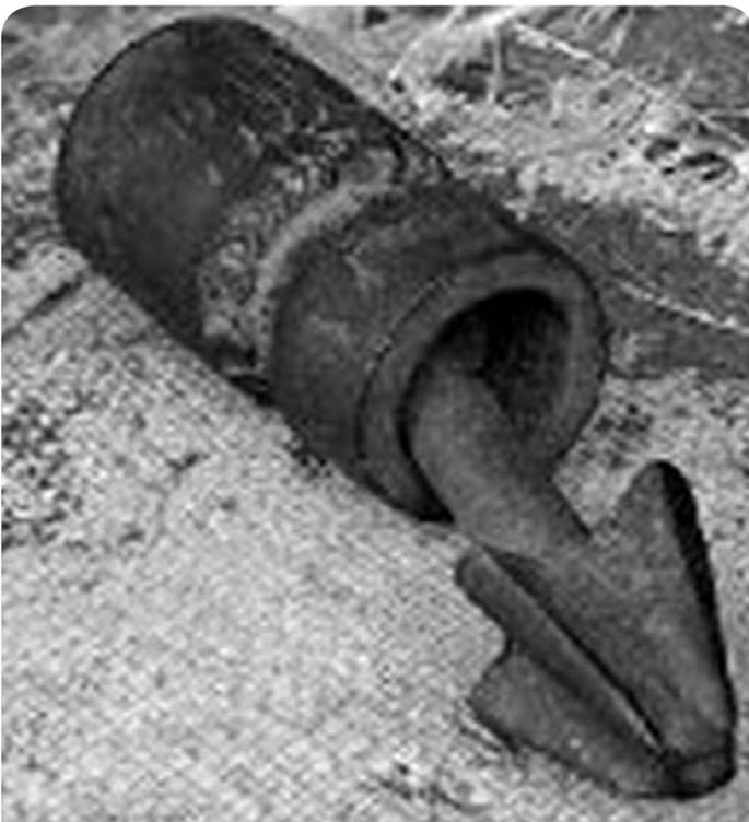
Fig. 2.25 Drill bit with footvalve above
