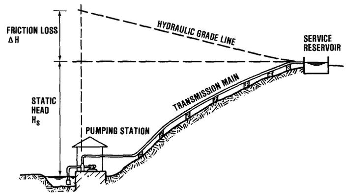
Fig. 4.25 Pressure in pipe
