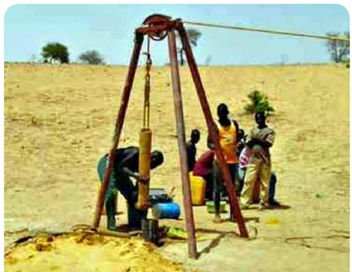
Fig. 2.16 Hand percussion rig in action
