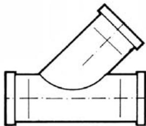
L) Tee 45°, equal female threads, galvanized
