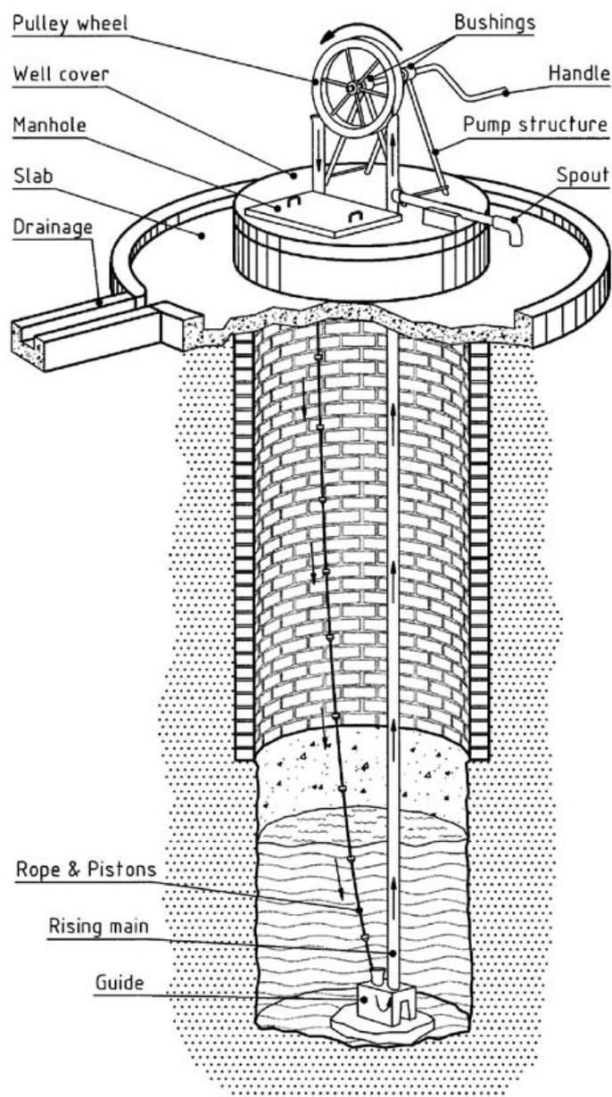
Fig. 1.6 Rope pump installation
