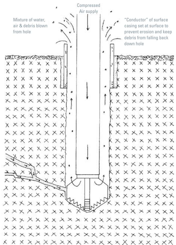
Fig. 2.37 Boreholes in consolidated rock
