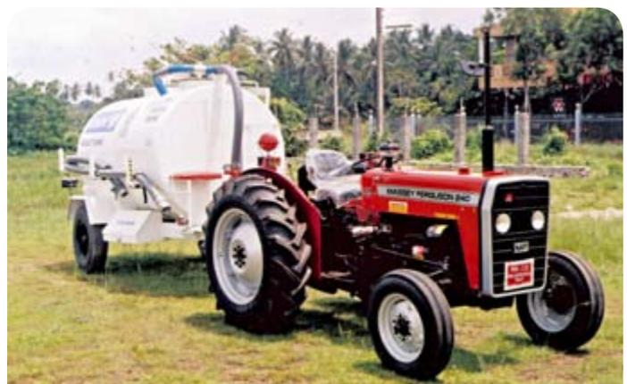
Fig. 5.7 The Sri Lankan tractor-drawn trailer-mounted vacuum tanker
