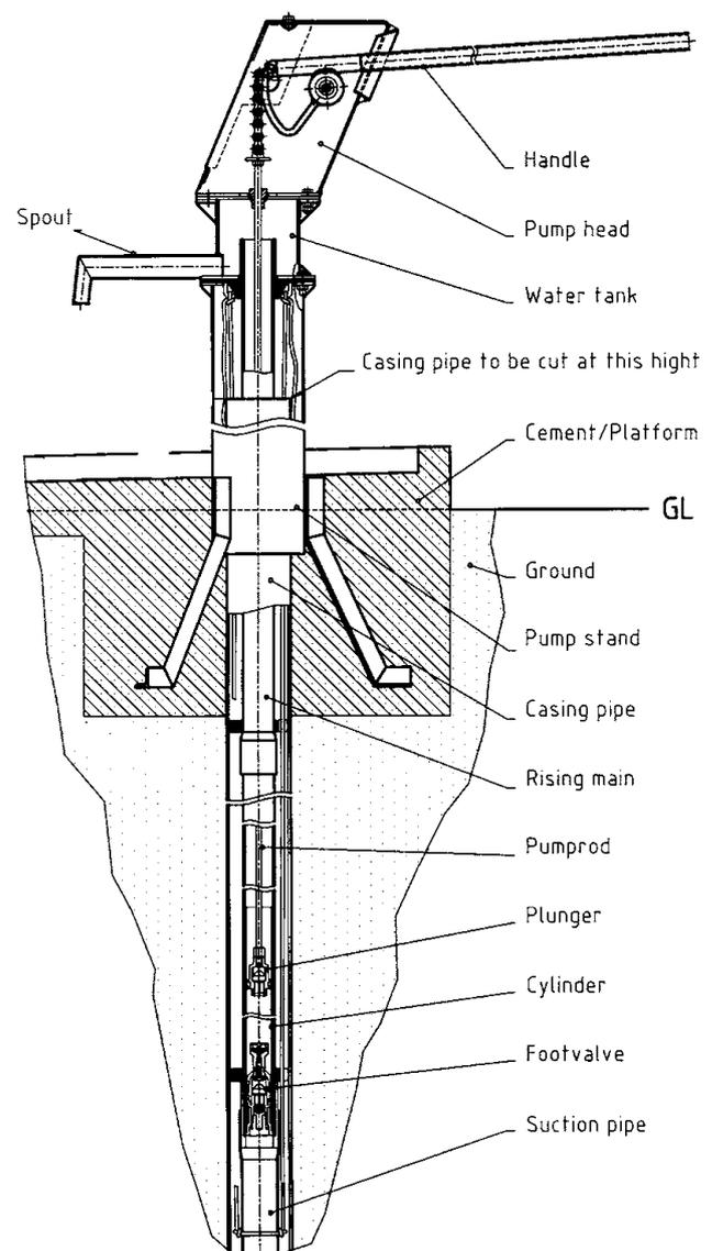
Fig. 1.43 U3M pump assembly
