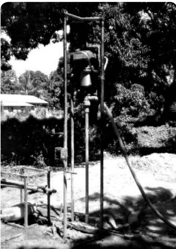
Fig. 2.61 Small rig with petrol engine drive, Tanzania © Skat
