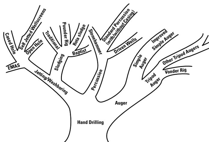
Fig. 2.12 Hand drilling family tree
