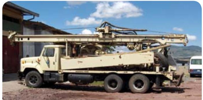
Fig. 2.62 Large hydraulic rotary rig, Ghana
