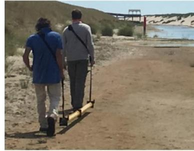
DUALEM 421, fixed frequency and 6 fix distances and orientations, Expl.Depth: upto ca 6m
