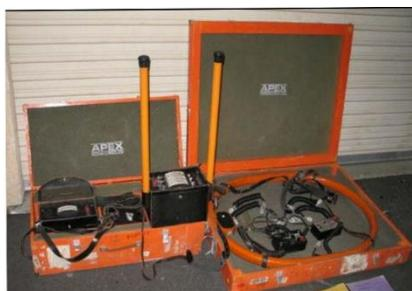
APEX MAXMIN, multi frequency EM, (out dated system), expl Depth upto ca 40 m, (depending earth resistivity)
