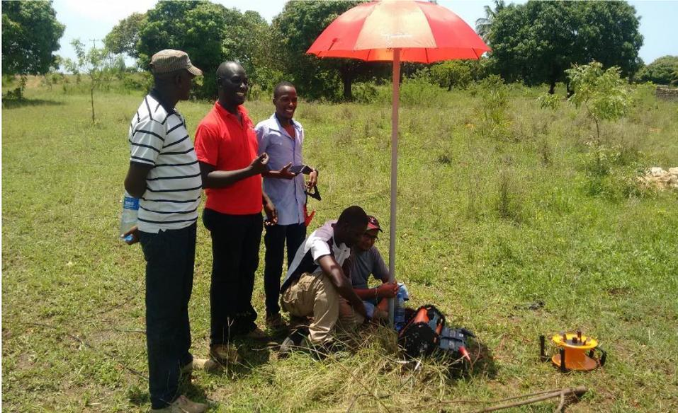
*Figure 23, demonstration of a WalkTEM sounding in Kwale, Kenya, only one person could handle this set up (40 X 40m) transmitter loop, exploration depth up to 150m.*
