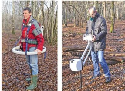
Iris Promis, multi spacing, multi frequency, 3 components of the secondary EM field (modern system) Expl. Depth upto ca 100 m (depending earth resistivity)
