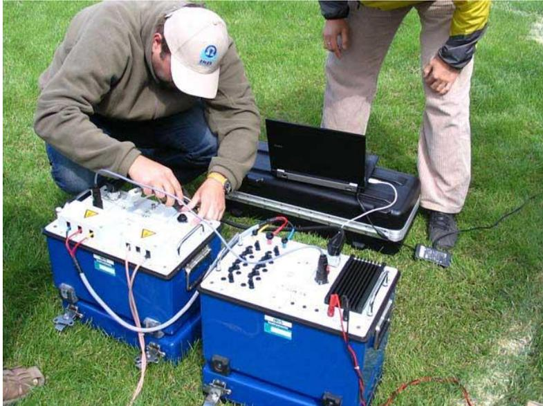
Figure 46, instrumentation of the IRIS numis light version (loop size 60 m, depth ca 50 m)
