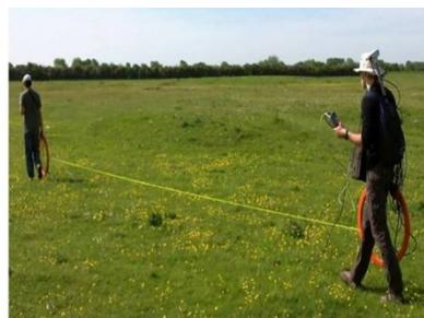
EM34, geonics, 3 antenna spacings, with fixed frequency's expl depth, upto ca <10, 20, 30 m (depending earth resistivity)
