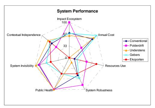
Figure 2: Example of the system performance benchmark: comparison of the conventional wastewater management system with 3 cases with urine separation in Sweden and 1 in the Netherlands
