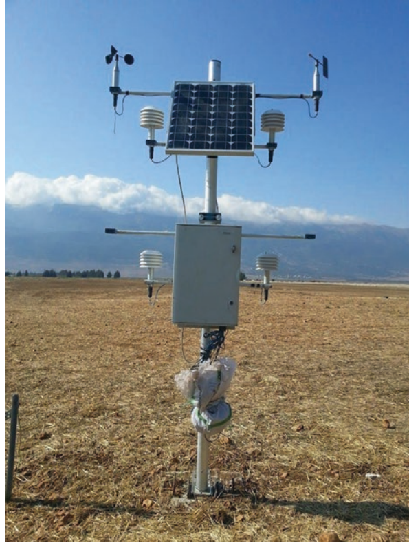
Fig. 2.3 Bowen ratio station (NESA) installed in the potato field
