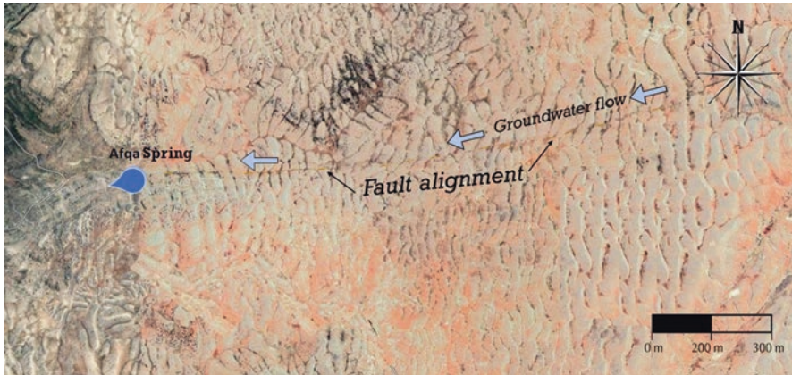
Fig. 4.4 Fault alignment transporting groundwater to Afqa Spring
