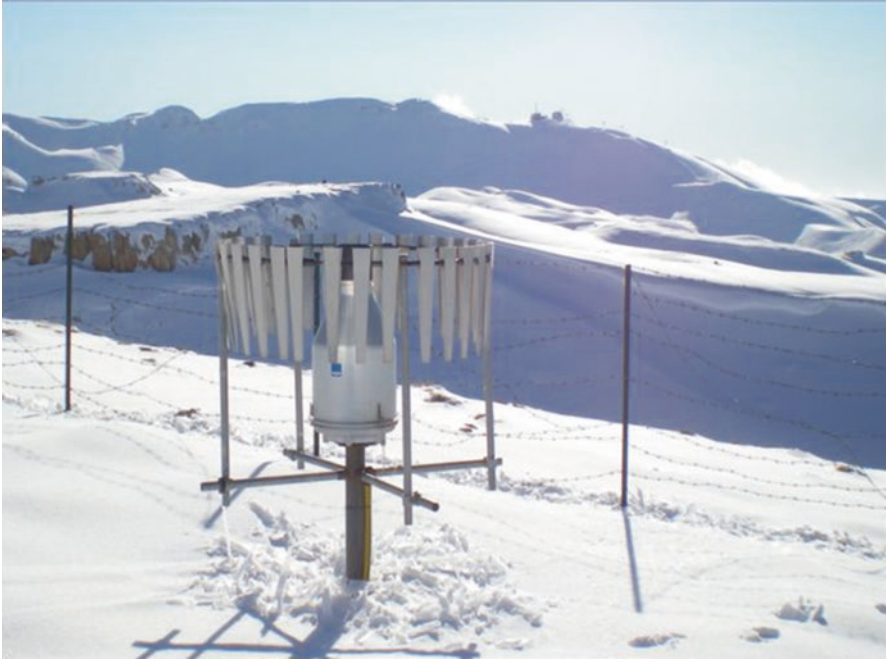
Fig. 5.1 Automated weather station for snow measuring in El-Mzar area, Mount-Lebanon
