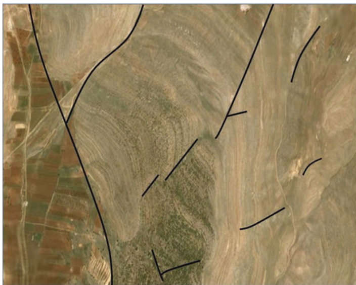
Fig. 8.4 Example showing the identified faults (black color) on Aster satellite image
