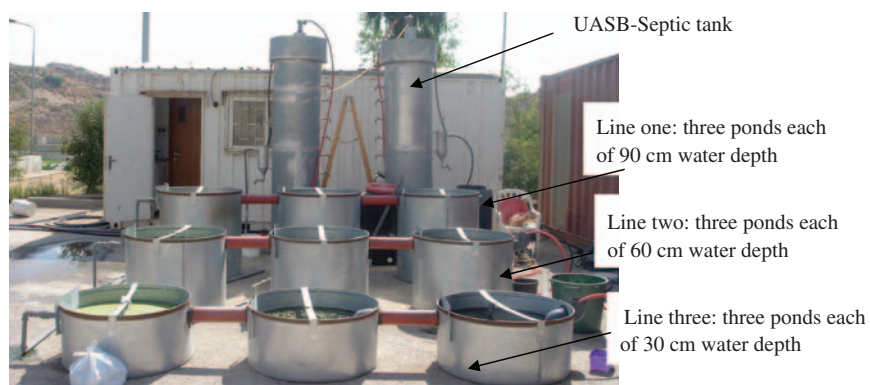
Figure 12.1 Photograph of the experimental pilot plant; the three lines of stabilization ponds and the UASB-septic tanks
