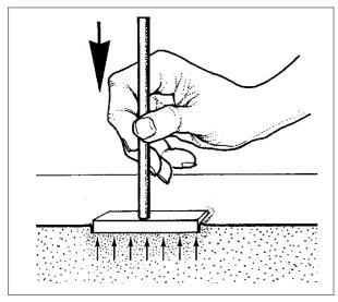
According to the weight of the structure and the type of the soil the size of the foundation needs to be designed. At too small foundation cannot be used in a low capacity bearing soil, it will sink into the soil.
