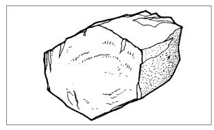
Stones built between corner stones are called line stones. They should be (but not necessarily) plain surfaced. The combination of plain surface corners and rough hammer dressed line stones give the stone masonry an attractive appearance.
