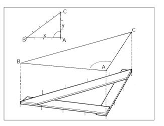
right angle is found at point A formed by the lines x and y.
