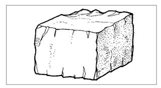
The two faces should be squared and shaped with chisel and club hammer to a plain surface, or at least hammer dressed to make accurate plumbing possible.
