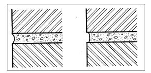
Made with pointing tool or a piece of small pipe. Two centimeters of the set mortar is scratched out of the joints and later filled with pointing mortar of a ratio 1:3 to 1:2 as shown in the drawing. This pointing is work intensive and expensive, but has a big influence on the quality of the structure.
