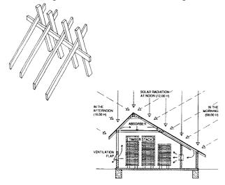
Kiln drying achieves accelerated seasoning in closed chambers by heating and controlling air circulation and humidity, thus reducing the drying time by 50 to 75%, but incurring higher costs. An economic alternative is to use solar heated kilns.
