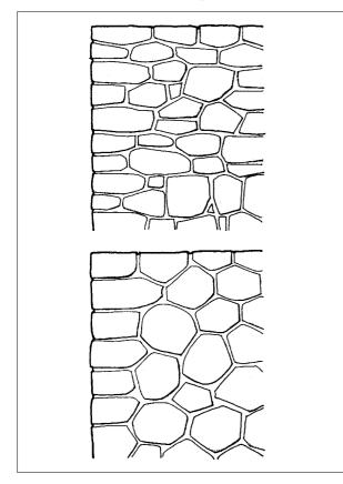
Uncoursed rubble masonry needs relatively little shaping and less precise jointing work. The layout and building of the structure will show clearly the builder's skill. Therefore, it is important to train builders in the special subject of stone masonry work. This kind of stone masonry uses all sizes of stones whose faces, joints and beds are roughly shaped. No attention is given to maintain level courses.
