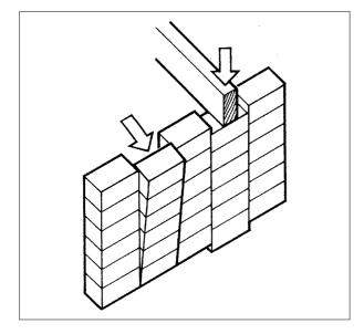
Bonded walls provide stability and resistance to the side thrust, as seen in the figure above. The bond can be selected to give an attractive appearance to the wall face.
