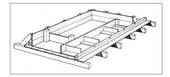
All form work material (planks, boards, steel etc.) and element form work (moulds) are sprinkled with water before placing concrete. After striking or dismantling, the form work is cleaned and eventually oiled as well as properly stored and protected from sun and rain. This will guarantee the use of many times.
