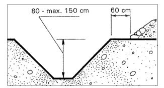
loose ground correct excavation
