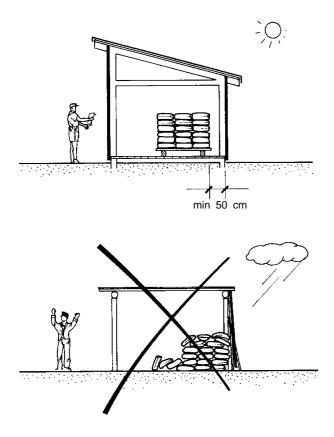
This is especially important in humid climates. The old stock should always be used before the new one. Cement can be expected to lose from its potential strength because of storage time as follows:
