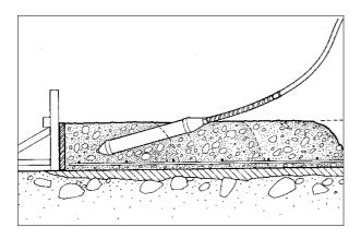
ment, to avoid vibration on the formwork or reinforcement. The vibration can cause holes and therefore weaken the structure.
