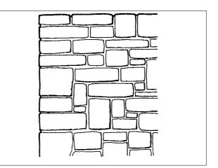
The rules for plumbing and lining are the same as for brick laying. It is advisable to hang one line for the inner wall and to work with two masons at the same time. One mason builds on the outside, the other on the inside of the line.
