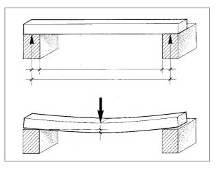
By embedding steel bars in the concrete, advantage is taken of these properties to improve the load carrying capacity of the structure. The steel is placed in the concrete that is subjected to tension but also to avoid cracks due to shrinking.
