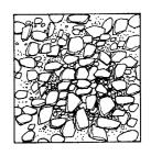
If possible use coarse grained sand and never the fine sieved sand used for masonry work. Remainders of coarse sand from sieved masonry sand can be added to the aggregates when mixed with coarse grained sand.
