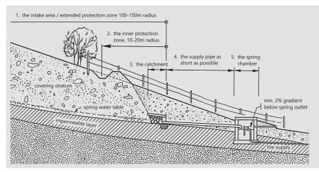
Figure 6: The five components of a spring catchment<sup>1</sup>
