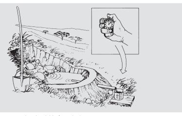
Figure 5: Measuring the yield of a spring<sup>1</sup>
