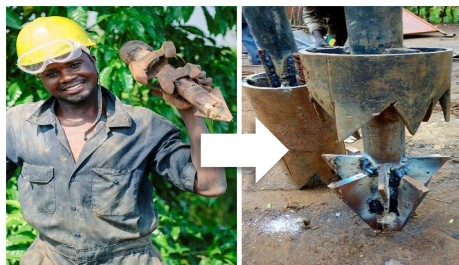
Drill bit of the jetting toolkit from Chad
