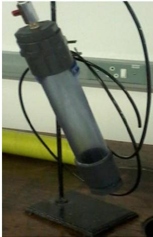
FIGURE 6. CAPILLARY EXTRUDER
