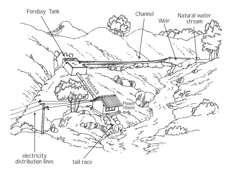
Water from the river is channelled through a settling basin, which helps to remove sediments that could harm the turbine. The water then flows into the forebay tank where it is directed downhill through a pipe called a penstock. When the water reaches the bottom, it drives a specially designed turbine to produce the electricity. (Source:'Micro-hydro power: the basics', Practical Action, available at http:// practicalaction.org/?id=micro\_hydro\_faq)
