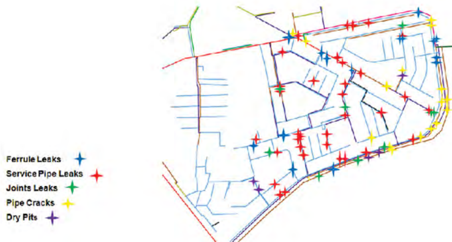
EXHIBIT 7.5: LEAKAGES IDENTIFIED AND MAPPED
