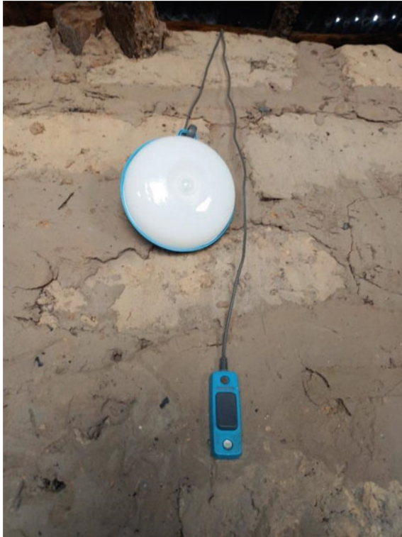
Fig. 3.4 An example of a solar lamp with a lease-to-own scheme (Note Users pay for electricity as they can, and eventually become owners of the system [Field Study in Southern Senegal, 2021])
