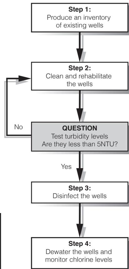
Figure 1.1. Steps for cleaning and disinfecting wells
