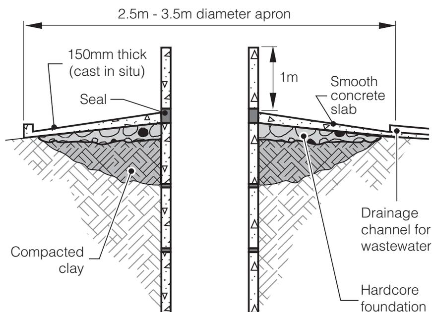
Figure 1.2. Sealing the top of a well
