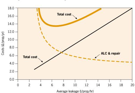
Fig. 6.1 Determining the economic level of leakage
