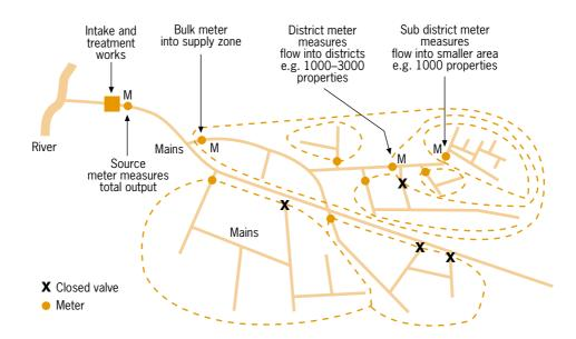
Fig. 7.1 shows a typical DMA design, including the monitoring hierarchy upstream and downstream of the DMA (reproduced from *Managing Leakage*—Report J).
