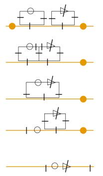
Fig. 8.3 A selection of meter and PRV installation layouts
