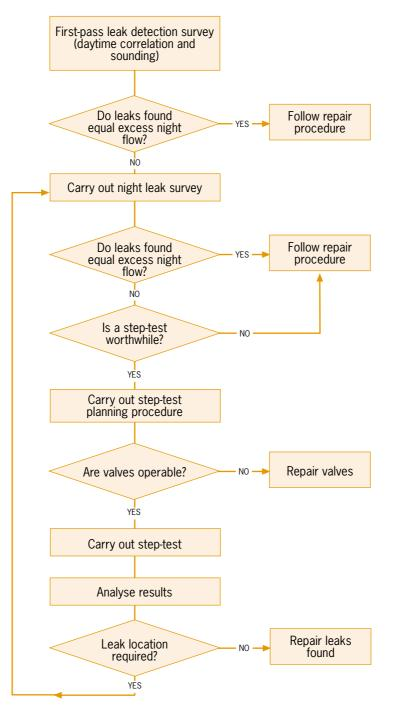
Fig. 9.7 A typical leak detection and location procedure
