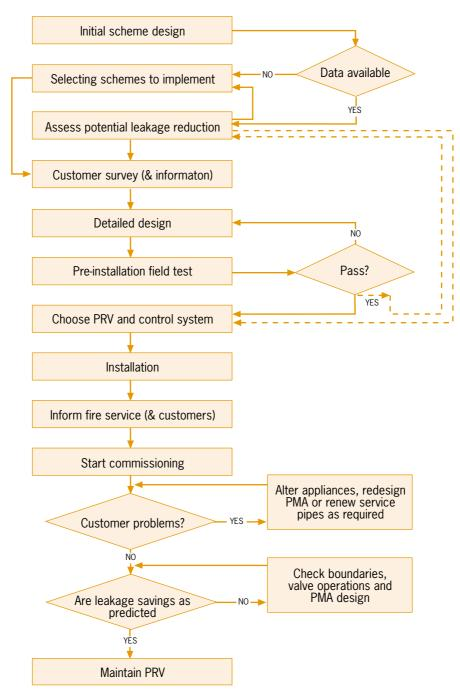
Fig. 8.1 Stages in PMA selection and design
