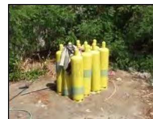
Chlorine cylinders stored under the sun; extreme heat may cause explosion
