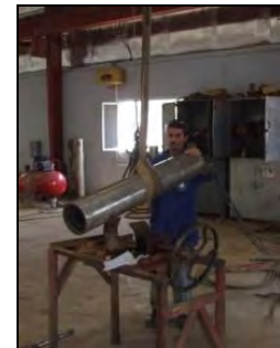
Working under or near overhead operations is dangerous because lifted items may fall; helmets are mandatory in such situations
