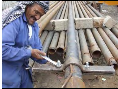
Wrong use of hand tools results in fatigue, and without proper hand protection
