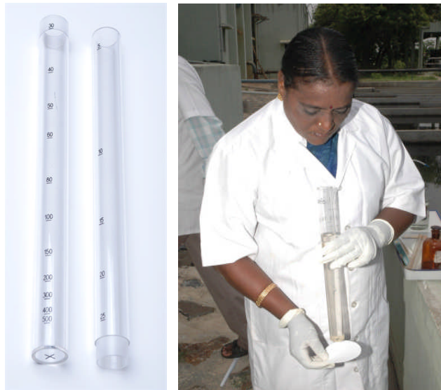
Figure 4.13 Use of a BOD tube for instantaneous assessment of the BOD at site.
