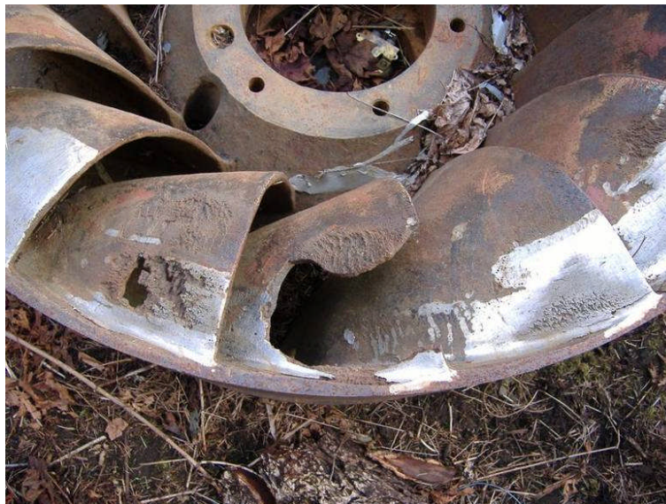
Figure 3.2 Typical cavitation damage of an impeller
