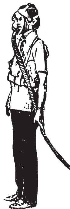
FIG. 6.16 AIR LINE RESPIRATOR
