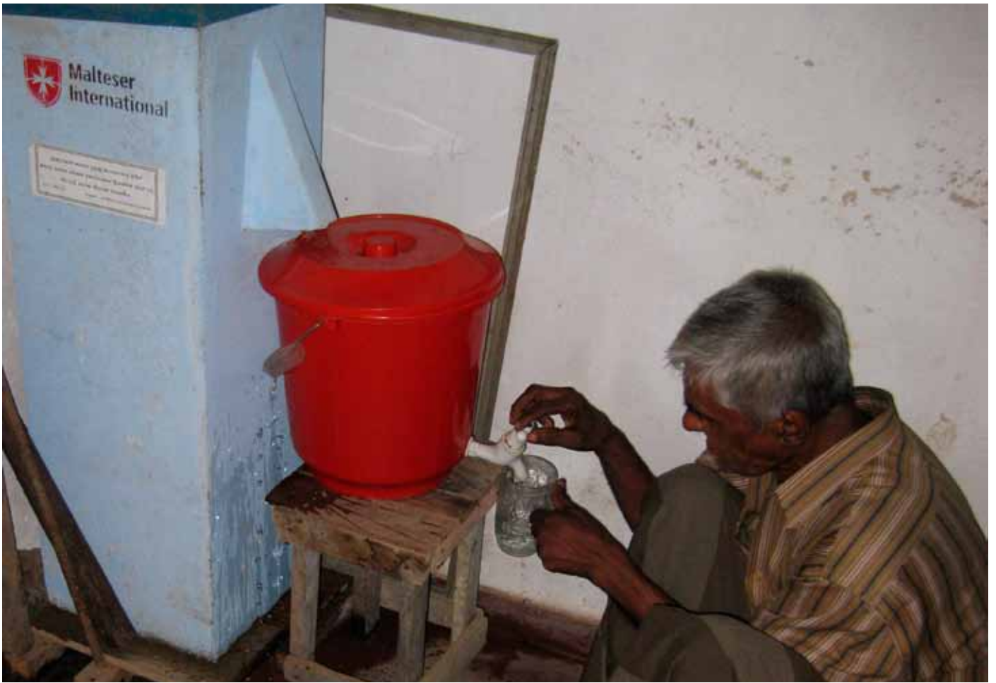
Hygienic management of drinking water at household level, Sri Lanka (Bio-sand filter)
