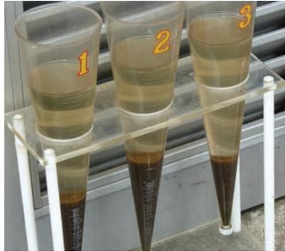
Figure 24. Imhoff cones. Perform sludge settleability tests with this inexpensive device.
