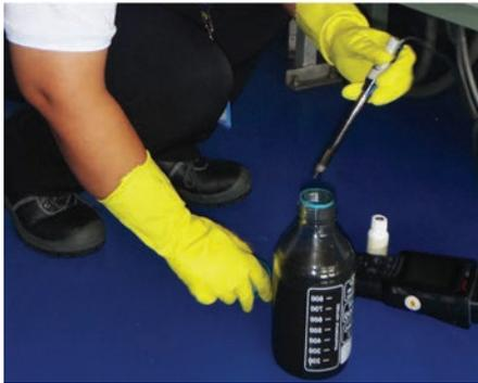
Figure 23. Checking the pH with a hand-held pH meter.
