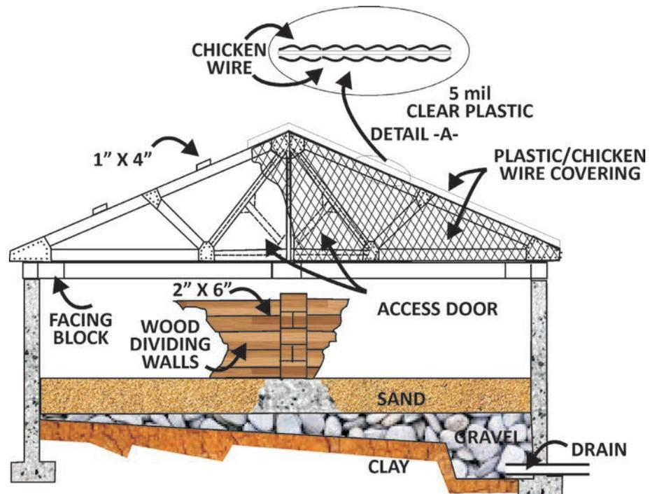
Figure 9. Underdrain system of a sand-drying bed.
