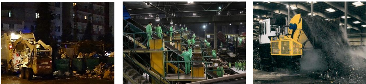
Figure 8 - Sukleen's system: (left) compactor truck collecting from overflowing bins, (centre) Qarantina sorting plant, showing manual sorting lines, (right) Coral windrow composting plant. Source: own picture (left), Sukleen 2015 (centre); CDR, 2014 (right).
