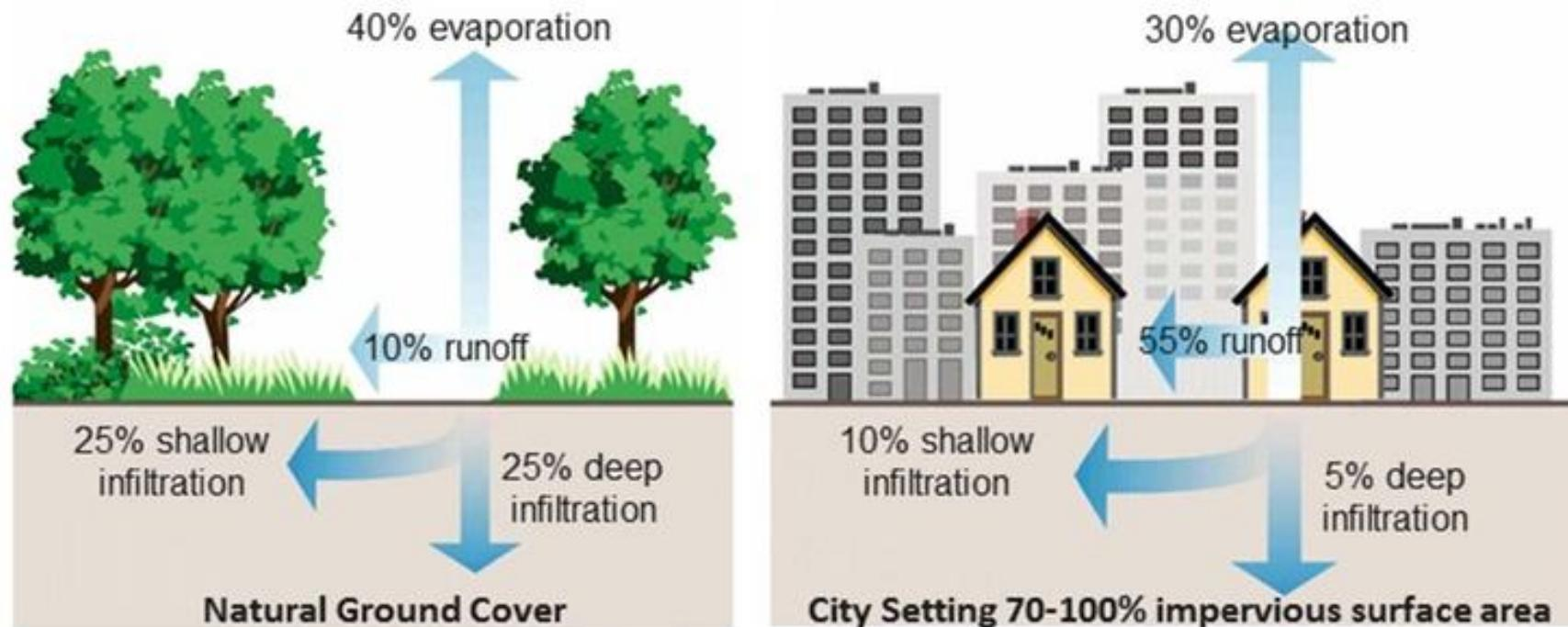
Stormwater infiltrates into the ground
