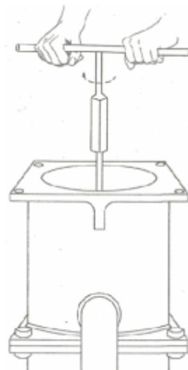
FAIRE TOURNER LA CLEF T DANS LE SENS D'UNE AIGUILLE D'UNE MONTRE, AINSI LE PISTON ET LE CLAPET DE RETENU SE REJOIGNENT.
