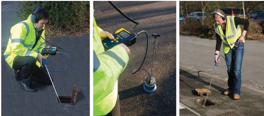
Figure 7.9 Electronic amplified listening devices. (Source: Primayer)
