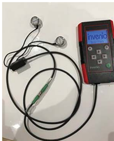
Figure 16.3 Vibration recorder. (Source: Invenio Systems)
