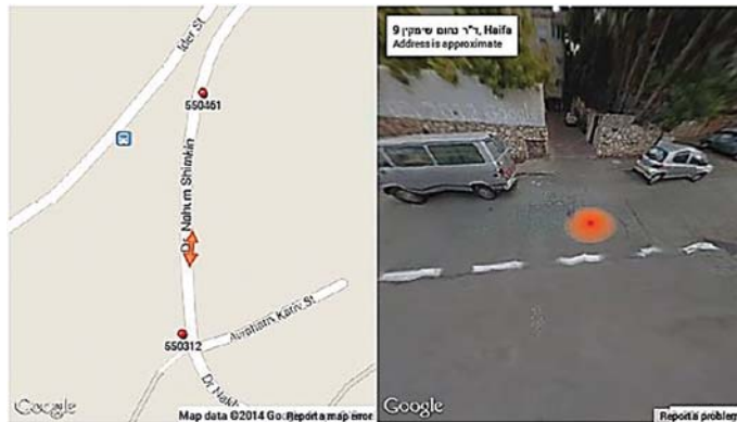
Figure 17.12.6 Leak position indicated in ZONESCAN NET. (Source: Gutermann)
