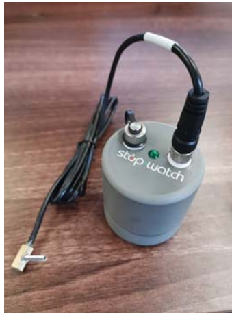
Figure 16.2 Device used for temperature measurements. (Source: Invenio Systems)
