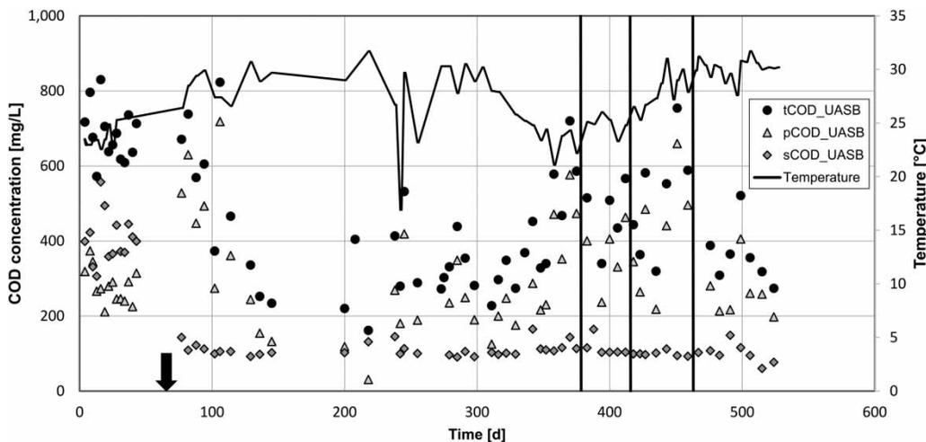
**Figure 5** | COD effluent concentrations of the UASB reactor (tCOD: total COD, pCOD: particulate COD, and sCOD: soluble COD) and effluent temperature. The arrow indicates the inoculation (day 65), the black lines represent the sludge removal.
