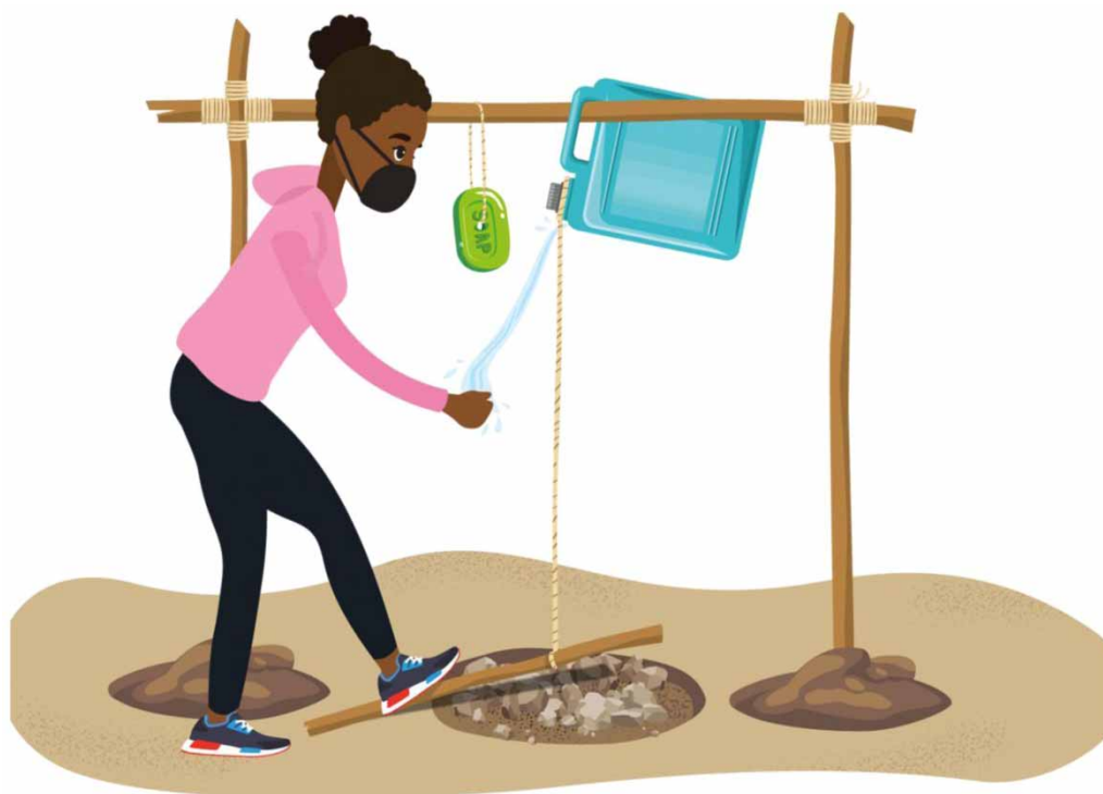
Figure 2 | Tippy-tap schema. Credit: UNICEF.
