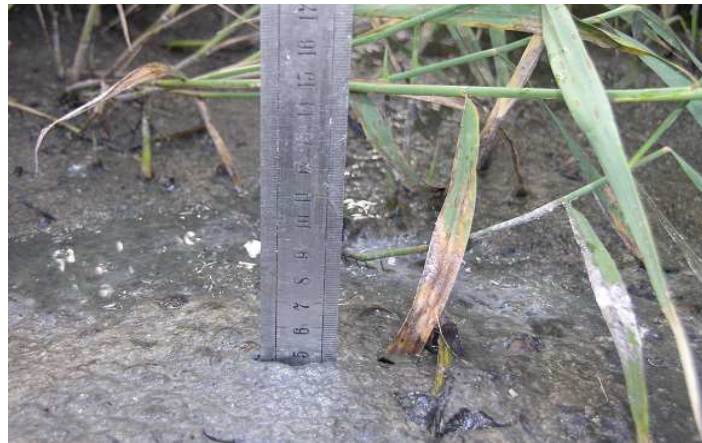
Measurement of the depth of the sludge accumulated in the first-stage
