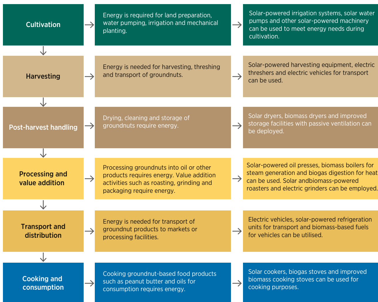
Figure 4 Energy needs at every stage of the groundnut value chain and the renewable energy solutions
