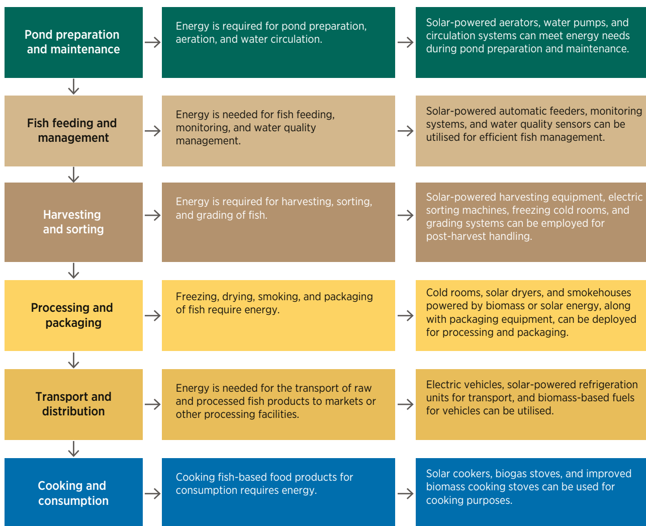
Figure 7 Energy needs at every stage of the fish value chain and the renewable energy solutions
