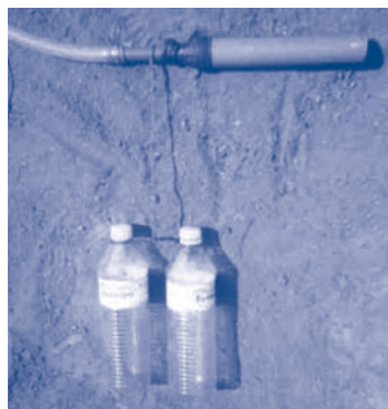
Figure 9.6. Ideal inlet and outlet arrangements (bottom-in top-out)
