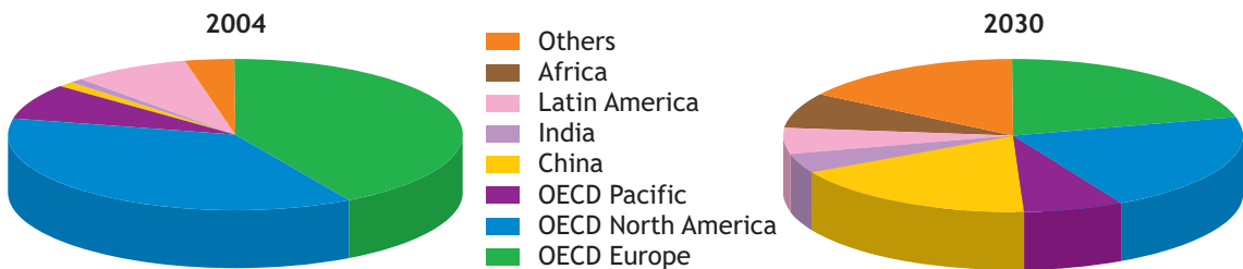
Figure 27 • Electricity from bioenergy CHP in 2004 (225 TWh total) and projections to 2030 (983 TWh total) by region
