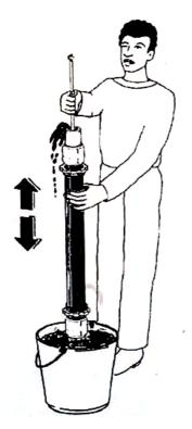
Place preassemble cylinder unit in a bucket filled of water.
