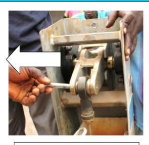
2) Remove the screw from the lever socket
