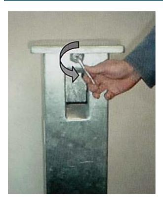
1) Unscrew Allen screw from pump body
