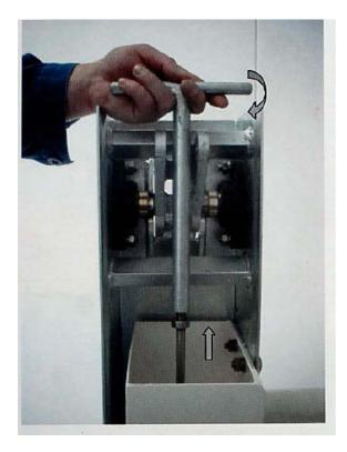
1) Screw T-bar onto the rod. Raise T-bar and lift the rod
