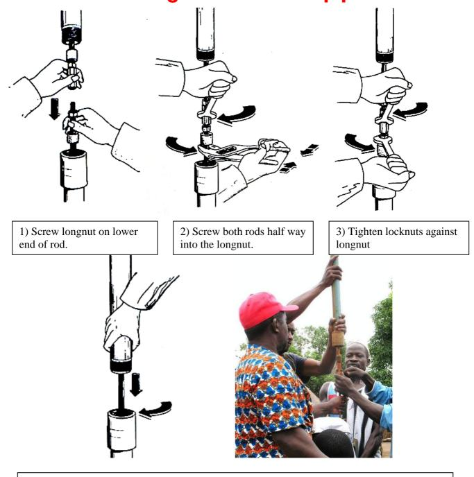
4) Screw riser pipe into double socket. Be careful not to damage the threads. Therefore, always hold riser pipe vertically. Screw slowly into double socket. Connect hand tight only
