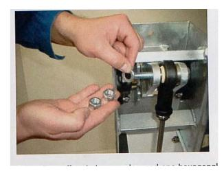
7) Take pliers off and place washer and one hexagonal nut on bolt
