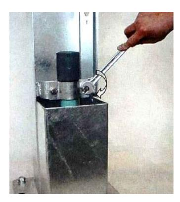
1) Push riser pipe and clamp into pump body and tight both screws
