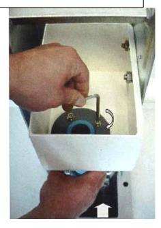
5) Tighten flange with screws and washers
