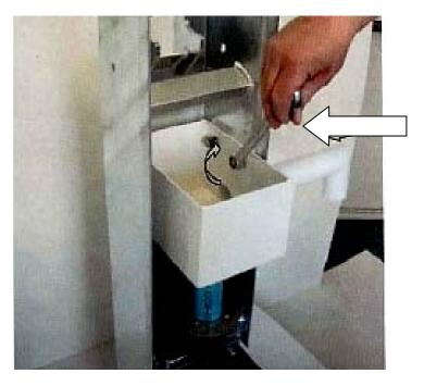
3) Unscrew the 3 screws of the water outlet pipe
