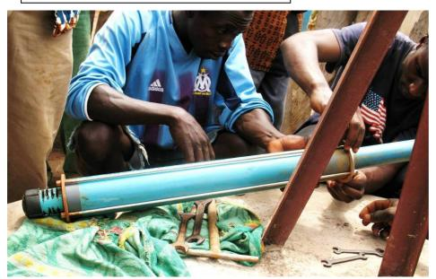
2) Make sure that all sealing rings are placed in their proper position
