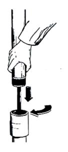
Unscrew riser pipe from double socket. Be careful not to damage the threads. Therefore, always hold riser pipe vertically
