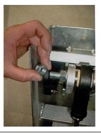
9) Place the second hexagonal nut on bolt and tighten it
