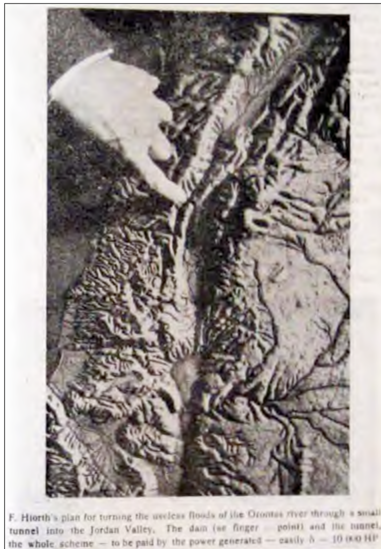
Figure 4.3 Hiorth's suggested plan to divert the Litani River into the Upper Jordan River, 1938 (Hiorth 1938: 29). The original caption reads "F. Hiorth's plan for turning the useless floods of the Orontes river through a small tunnel into the Jordan Valley. The dam (see finger — point) and the tunnel, the whole scheme — to be paid by the power generated — easily 5 — 10 000 HP". (It is in fact the Litani (not the Orontes) River that is both indicated and intended).
