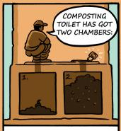
CHAMBER 1: IN USE CHAMBER 2: LOCKED TO PREVENT USE WHILE COMPOSTING IS IN PROCESS
