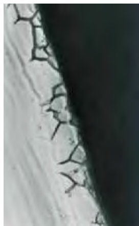
Intergranular corrosion of stainless steel
