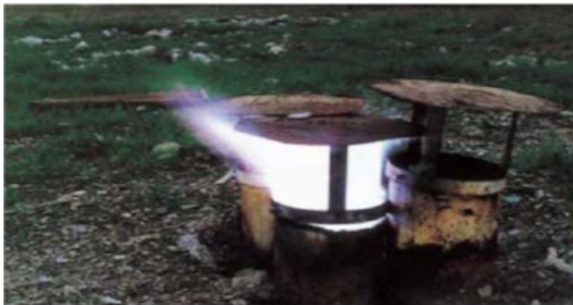
Landfill gas combustion test
